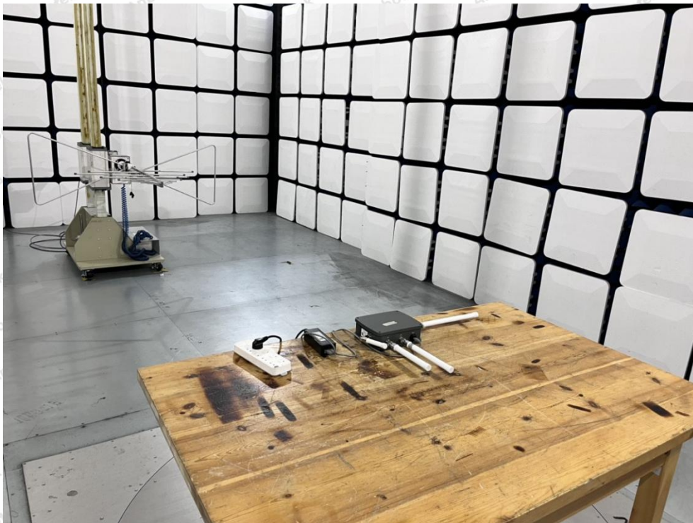
Photo of Radiation Emission Test
