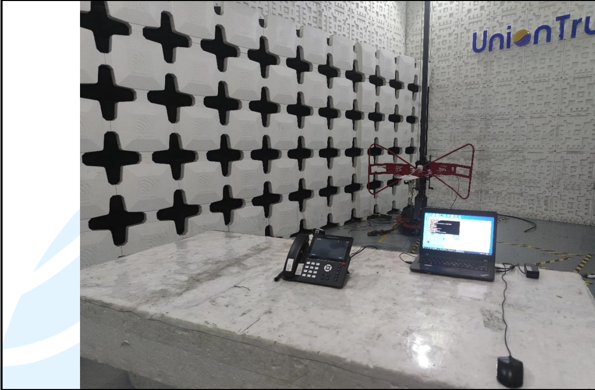
Radiated emission Test Setup (30 MHz~1 GHz)
