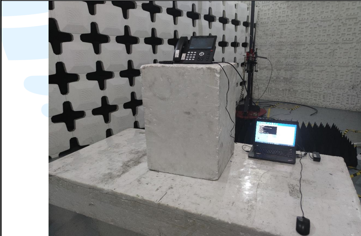
Radiated emission Test Setup (Above 1 GHz)
