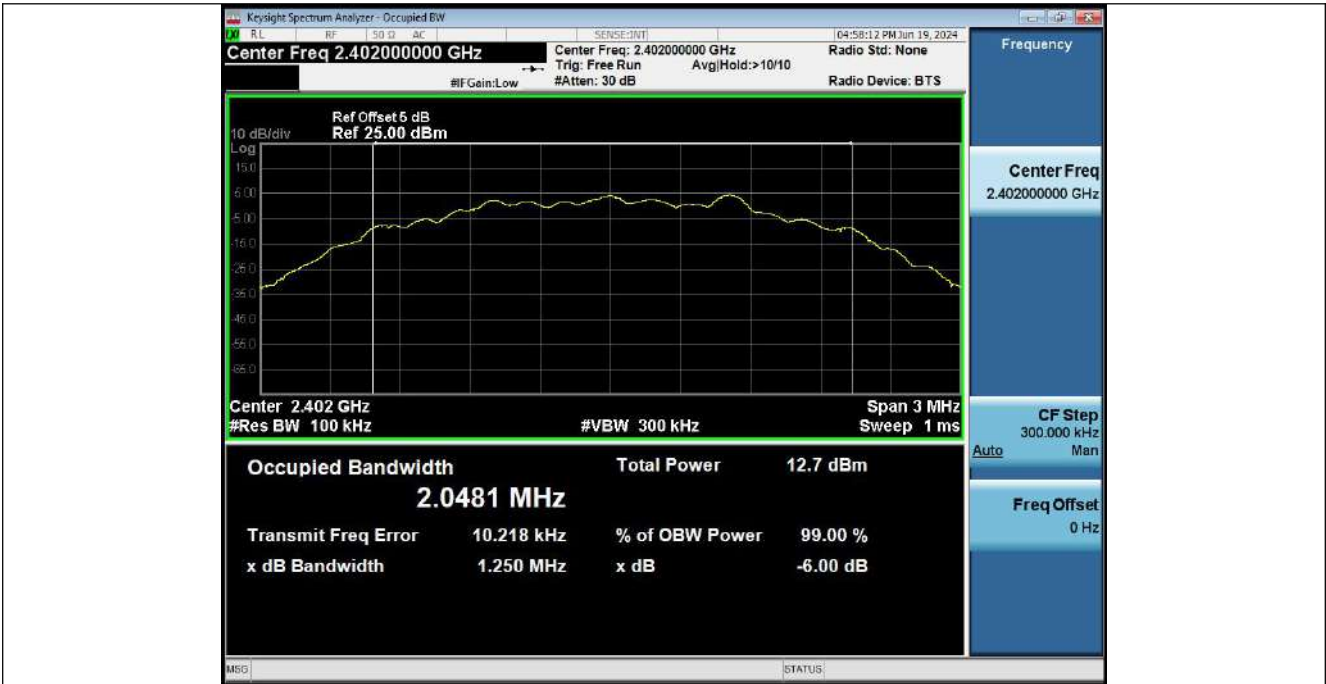
-6dB Bandwidth NVNT_ANT1_2Mbps_2440
