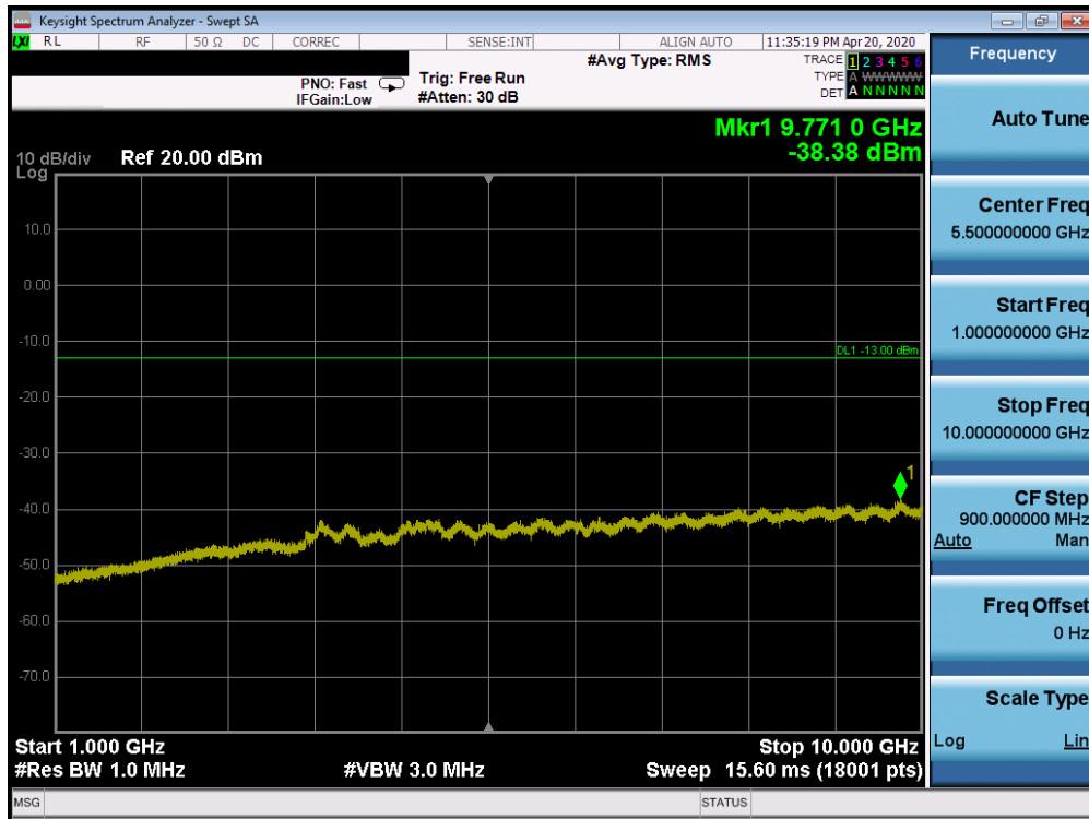
Plot 7-105. Conducted Spurious Plot (Band 12 - 10.0MHz QPSK - RB Size 1, RB Offset 0 - Low Channel)
