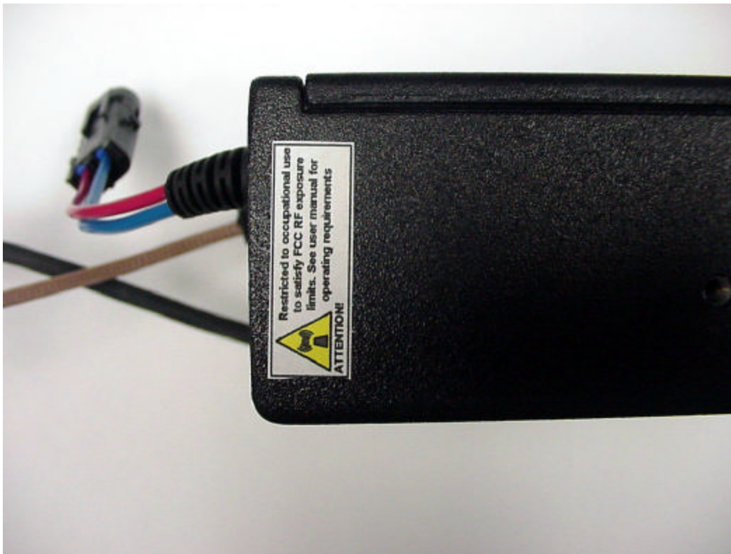
Radio side showing RF safety label
