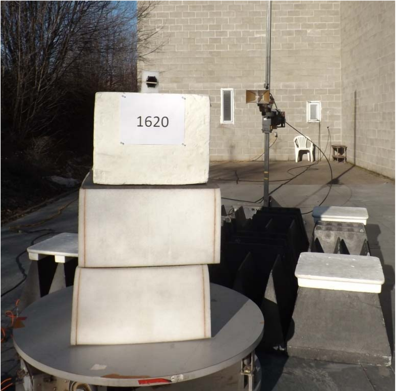
Figure E16.4 – Setup, Radiated Measurements, 1 – 18GHz
