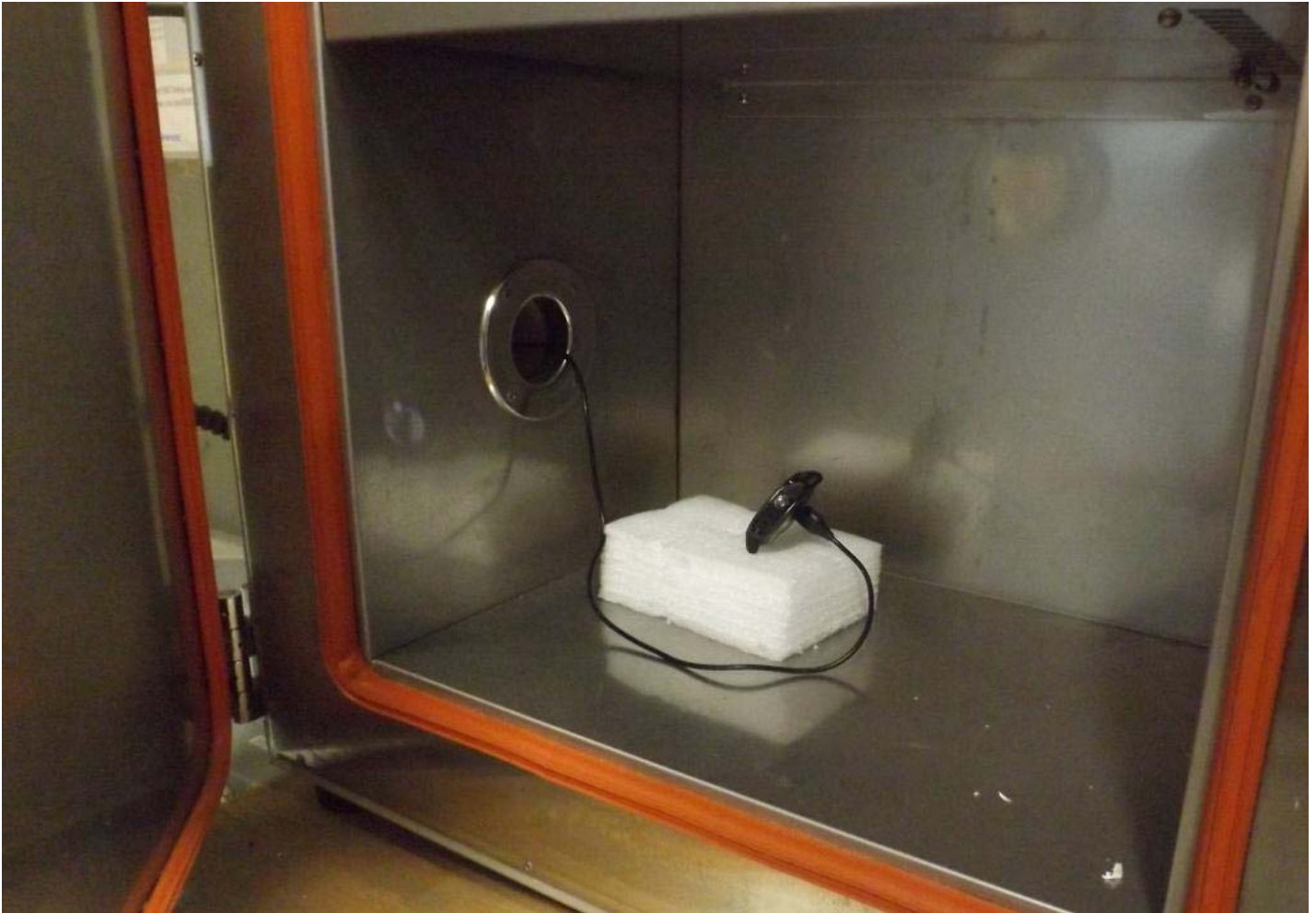
Figure E16.8 – Setup, NFC Frequency Stability Measurements
