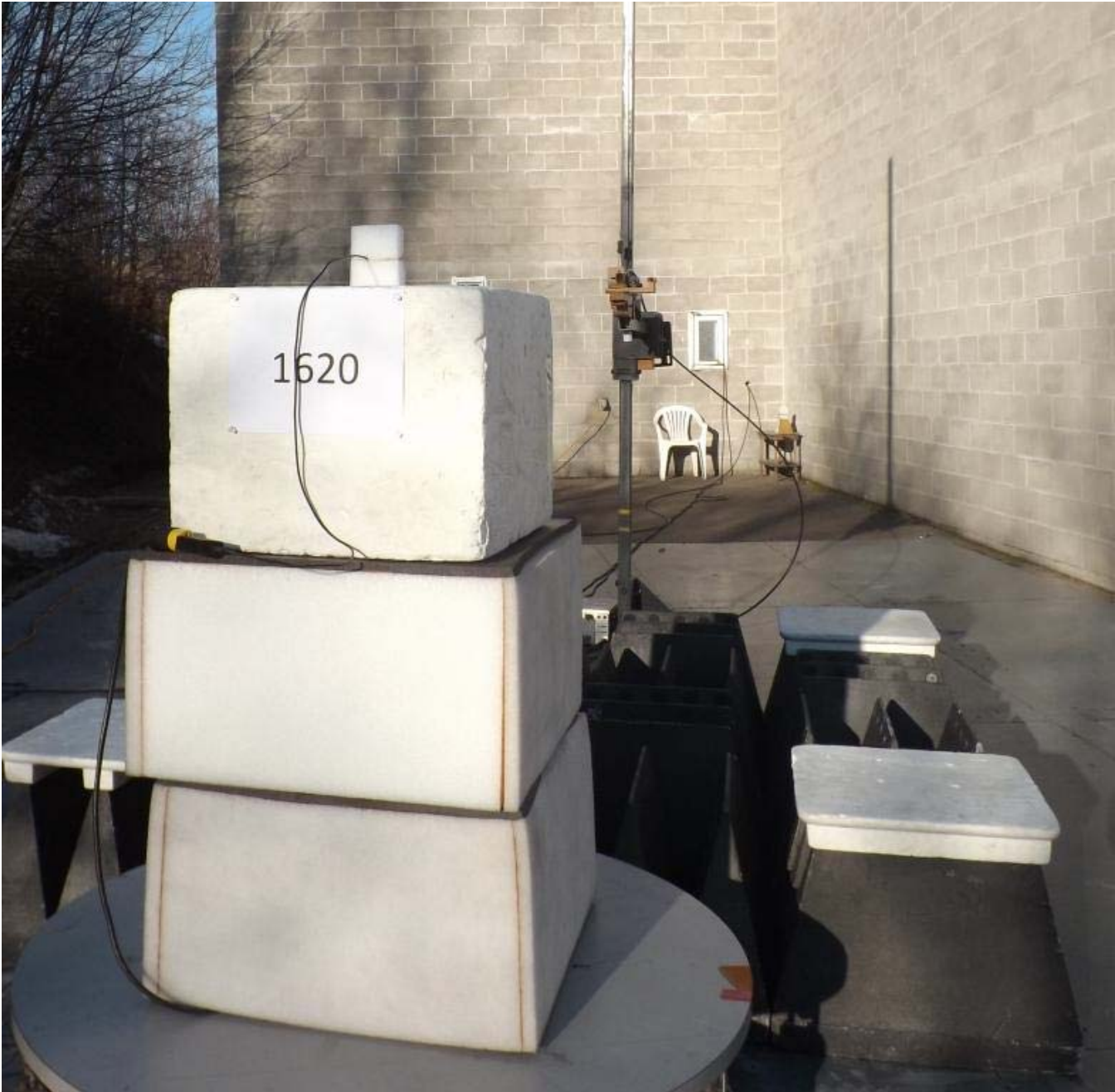
Figure E16.5 – Setup, Radiated Measurements, 18 - 26GHz
