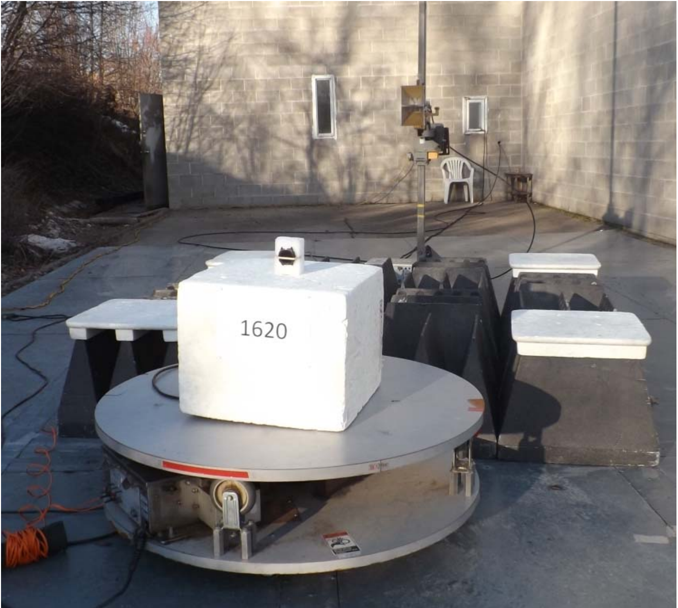
Figure E16.6 – Setup, Radiated Rx Measurements, 1 - 18GHz
