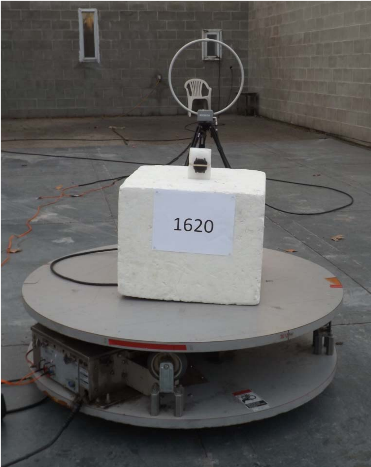
Figure E16.2 – Setup, Radiated Measurements <30MHz
