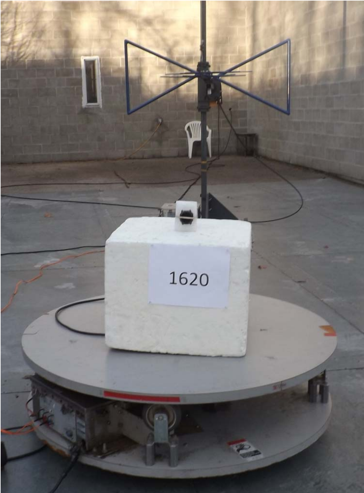
Figure E16.3 – Setup, Radiated Measurements 30 – 1000MHz
