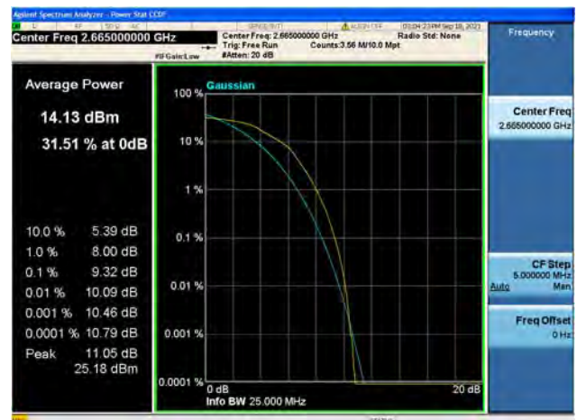
Band41 / 20MHz / High CH / 64QAM
