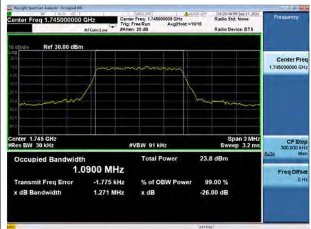
Band66 / 1.4MHz / Mid CH / 64QAM
