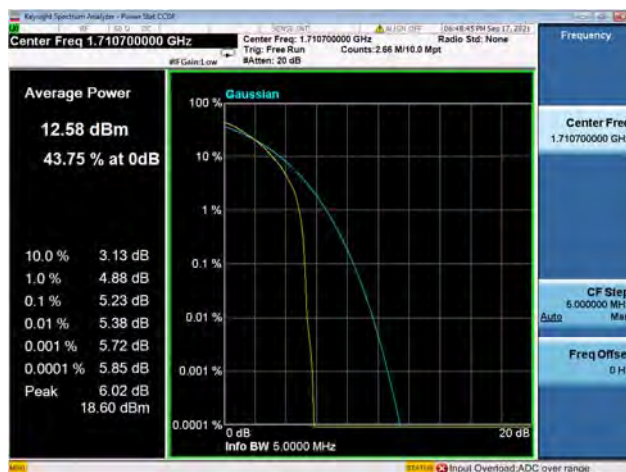
Band66 / 1.4MHz / Mid CH / 16QAM
