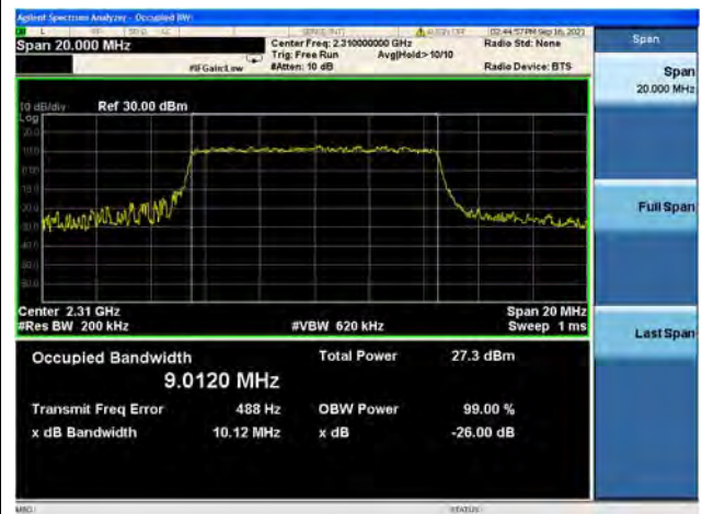
Band40/ Block A / 10MHz / Mid CH / 64QAM
