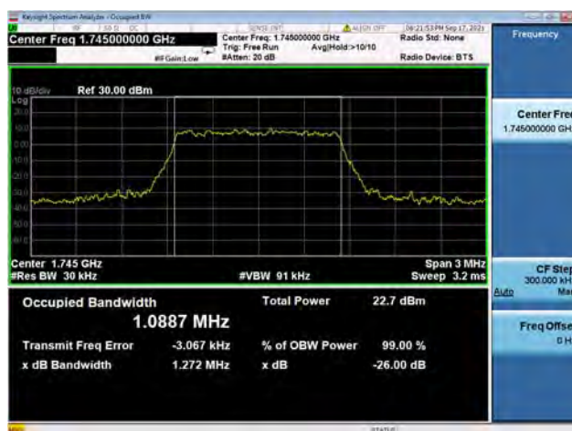
Band66 / 1.4MHz / Mid CH / 16QAM
