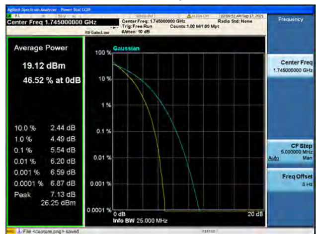
Band4 / 20MHz / High CH / 64QAM
