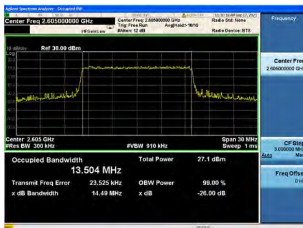
Band41 / 15MHz / Mid CH / 16QAM
