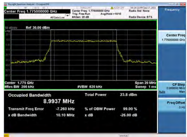
Band66 / 10MHz / High CH / 64QAM
