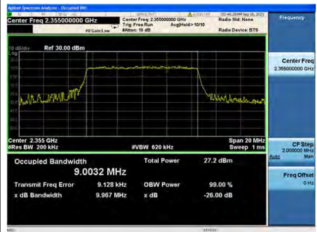
Band40/ Block B / 10MHz / Mid CH / 64QAM
