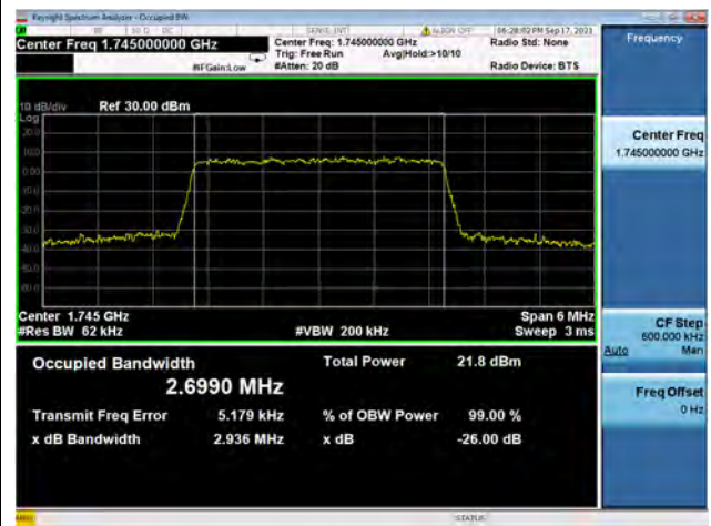
Band66 / 3MHz / High CH / QPSK
