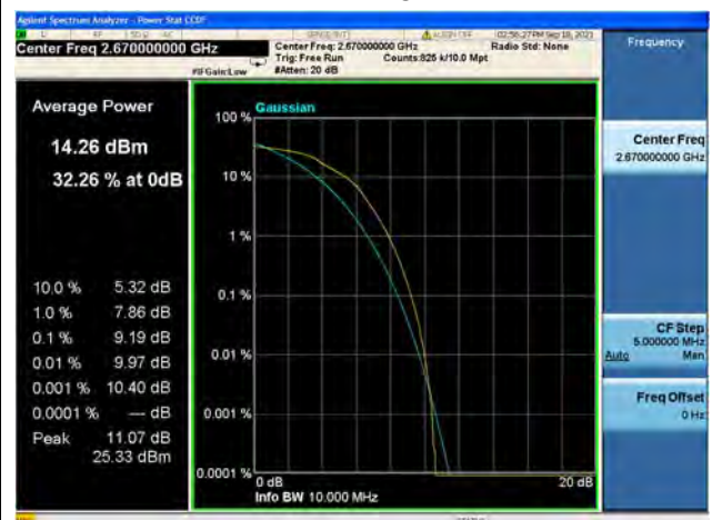
Band41 / 10MHz / High CH / 64QAM
