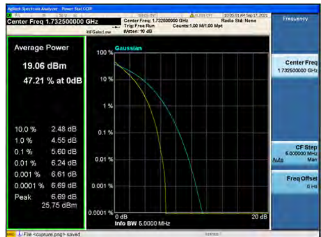
Band4 / 1.4MHz / Mid CH / 64QAM
