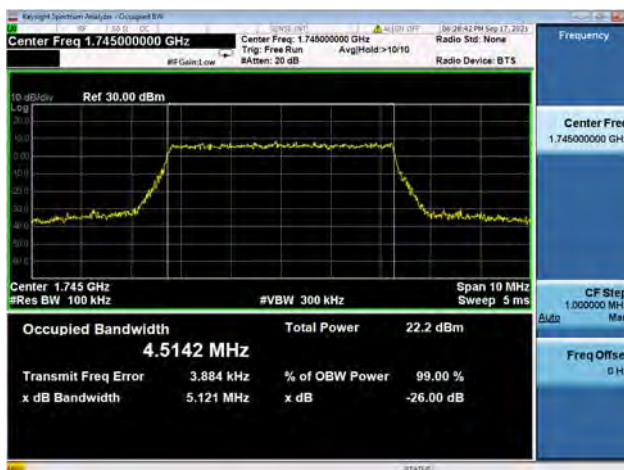
Band66 / 5MHz / Mid CH / 16QAM
