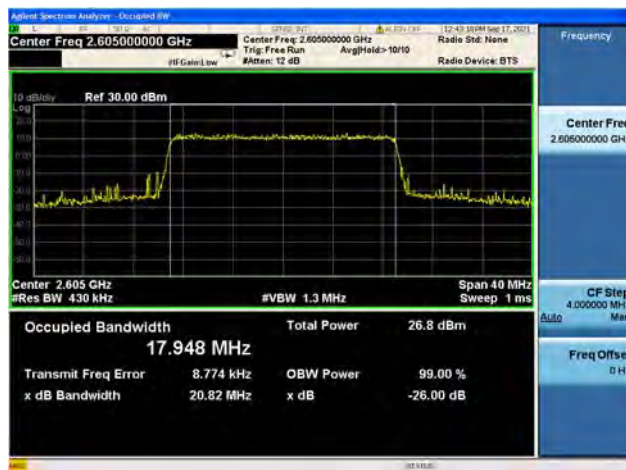
Band41 / 20MHz / High CH / 16QAM
