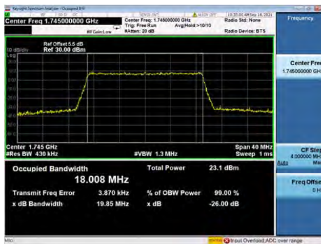
Band66 / 20MHz / High CH / 16QAM
