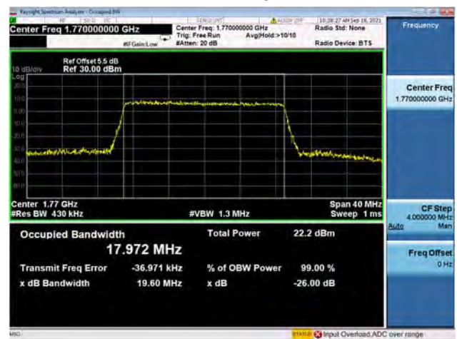
Band66 / 20MHz / High CH / 64QAM
