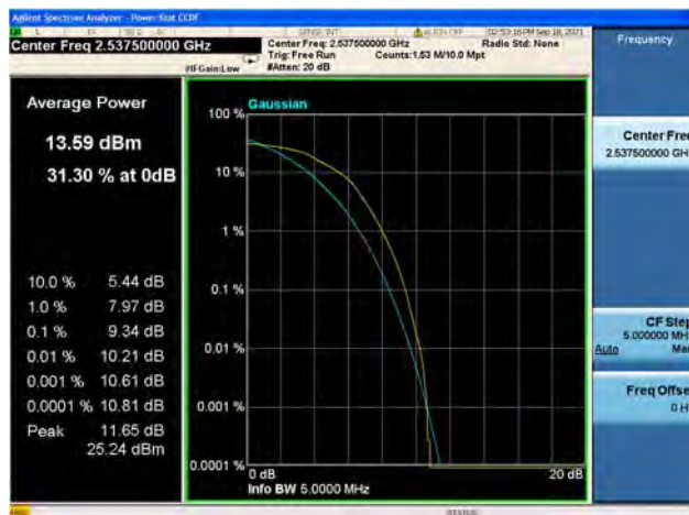
Band41 / 5MHz / Mid CH / 16QAM
