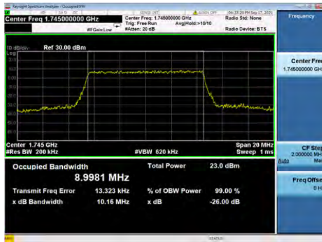
Band66 / 10MHz / Mid CH / 64QAM
