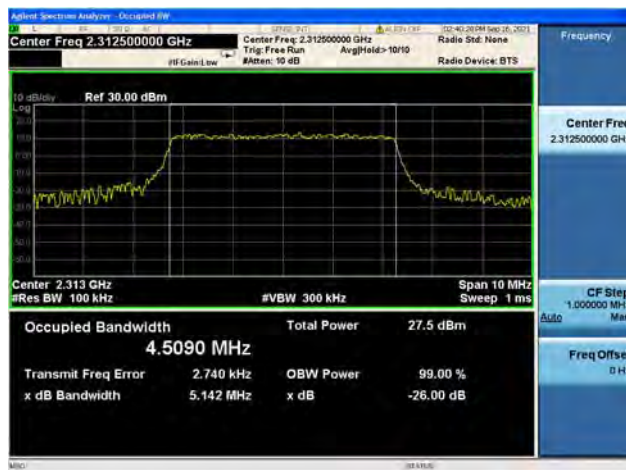
Band40/ Block A / 10MHz / Mid CH / 16QAM
