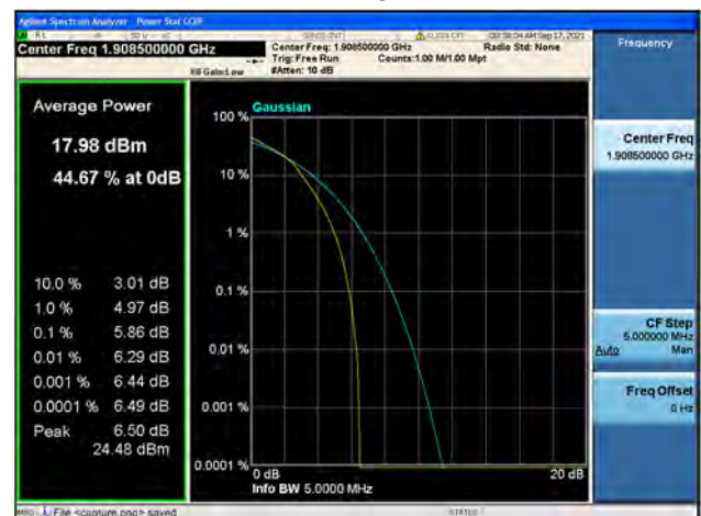
Band2 / 3MHz / High CH / 64QAM
