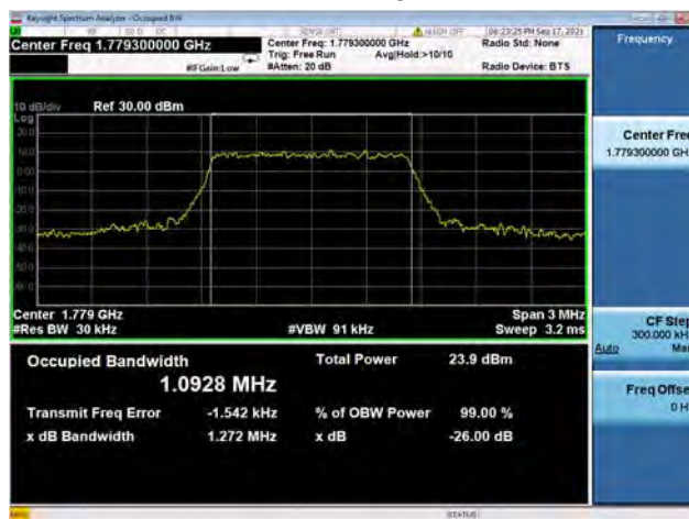
Band66 / 3MHz / Low CH / 16QAM
