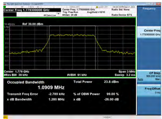
Band66 / 3MHz / Low CH / QPSK
