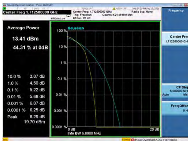
Band66 / 5MHz / Mid CH / 16QAM
