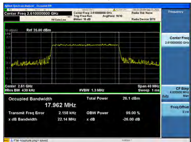
Band38 / 20MHz / High CH / 64QAM
