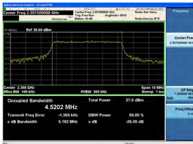
Band40/ Block A / 5MHz / Mid CH / 16QAM
