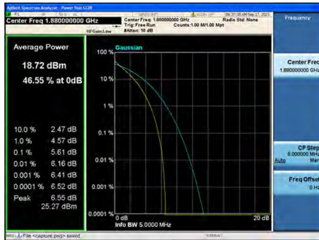
Band2 / 3MHz / Mid CH / 64QAM
