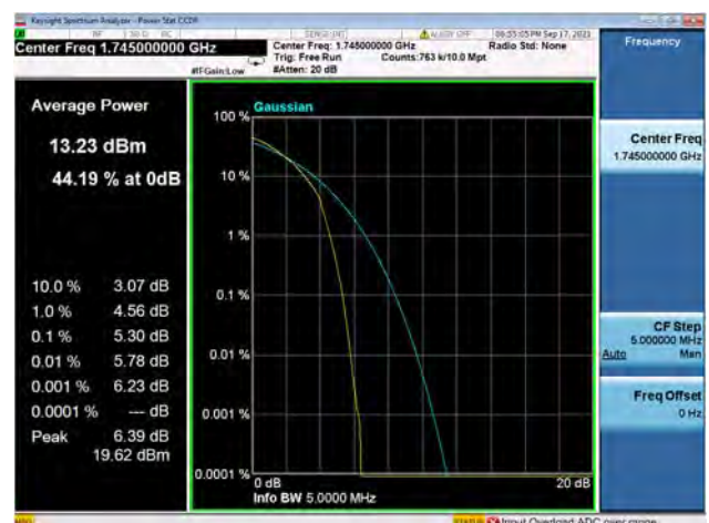
Band66 / 5MHz / Mid CH / 64QAM
