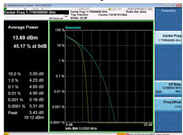
Band66 / 3MHz / High CH / 64QAM
