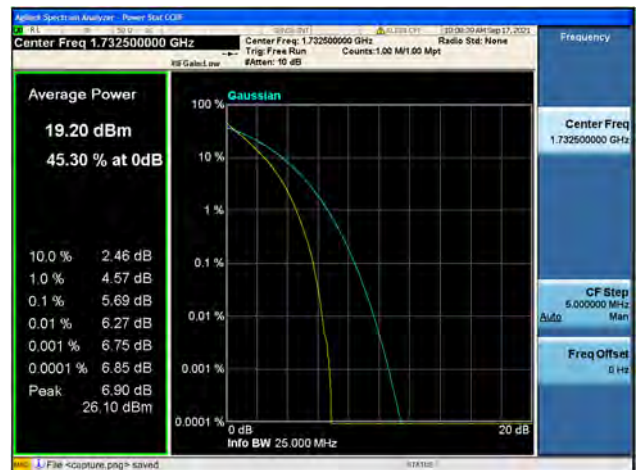
Band4 / 15MHz / Mid CH / 64QAM
