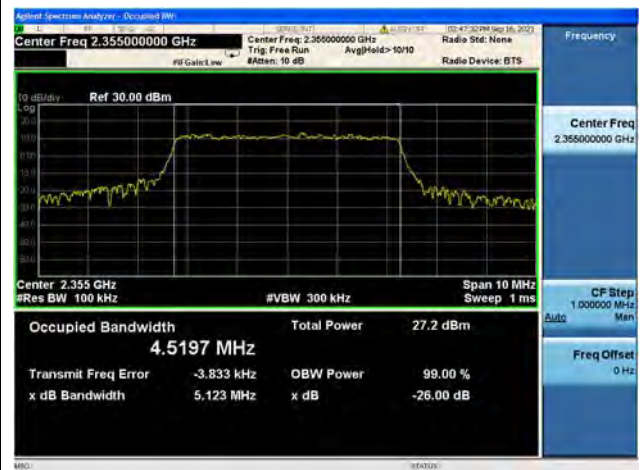
Band40/ Block B / 5MHz / Mid CH / 64QAM
