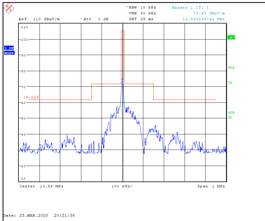
Figure 3 - Plot of the Fundamental 13.56 MHz
