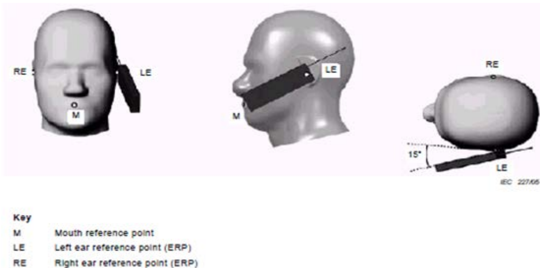
Figure 2 Tilt position of the wireless device on the left side of SAM
