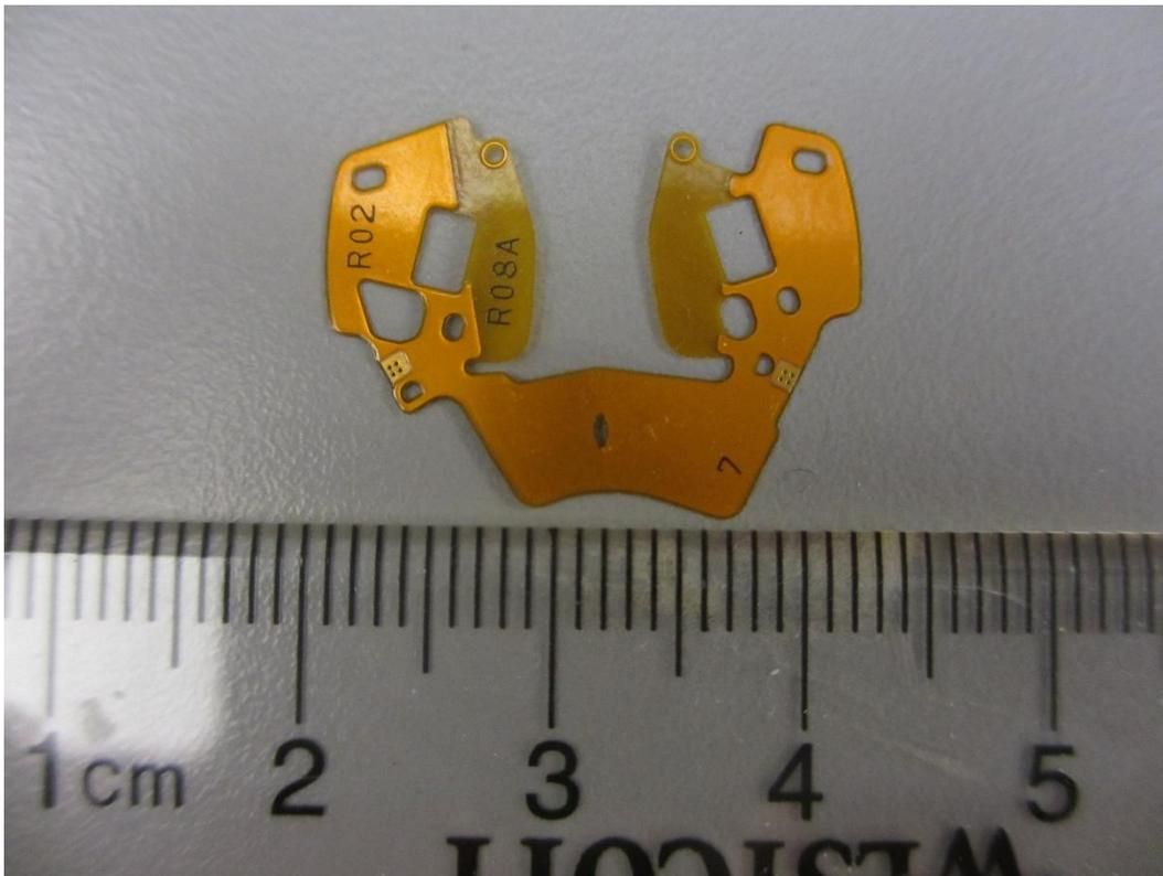
Figure 1 2.4 GHz Antenna (scale in cm)
