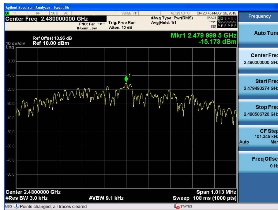
**9.6 OUT OF BAND EMISSIONS AT THE BAND EDGE/ CONDUCTED SPURIOUS EMISSIONS****Test Requirements and limit, §15.247(d) / RSS-247(Issue 2) Section 5.5.**
