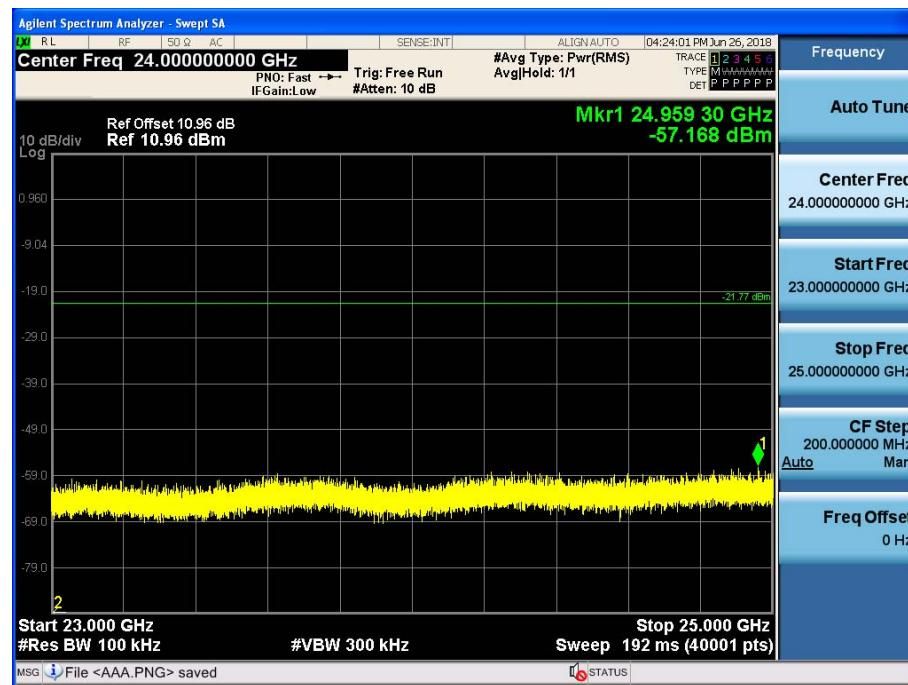
**9.7 RADIATED MEASUREMENT.****9.7.1 RADIATED SPURIOUS EMISSIONS.**
