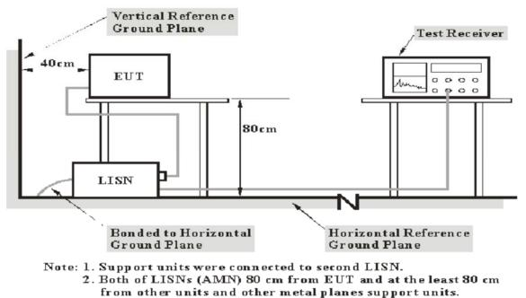
The setup of EUT is according with per ANSI C63.10-2013 measurement procedure. The specification used was with the FCC Part 15.207 and RSS-GEN limits.
