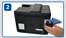
Remove the access cover from the printer.
