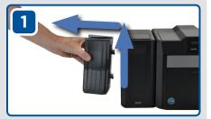
Remove the output bin from the dual side module (if attached).
