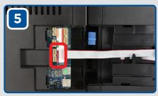
Connect the lamination cable to the printer connector (labeled pink).
