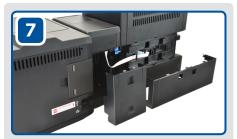
Replace the dual side module and lamination module access covers. **Note:** The dual side module cover must be rotated 180°.
