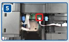
Connect the lamination cable to the connector on the dual side module.
