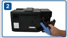
Remove the access cover from the dual side module.
