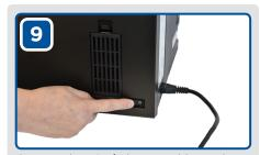
Connect the USB/Ethernet cables to the printer (as required) and switch on the printer.
