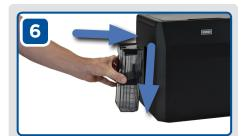
Attach the output hopper supplied with the lamination module. Do not use the output hopper supplied with the printer.
