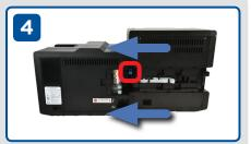
Move the blue lever on the lamination module down. Align the posts and slide the lamination module into place. Move the blue lever up to lock.
