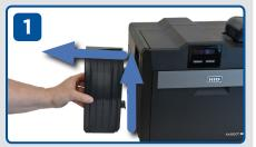
Remove the output bin from the printer (if attached).
