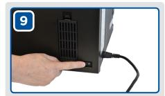
Connect the USB/Ethernet cables to the printer (as required) and switch on the printer.
