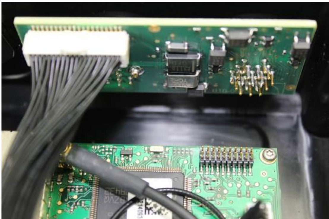
Figure 2 – Connector PCB Internal View
