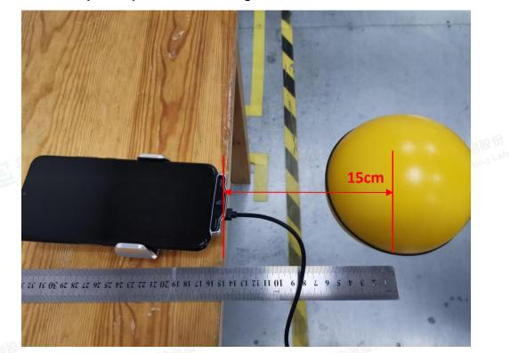
(TM1) Test Position B - Exposure photo from side edge surface-Left
