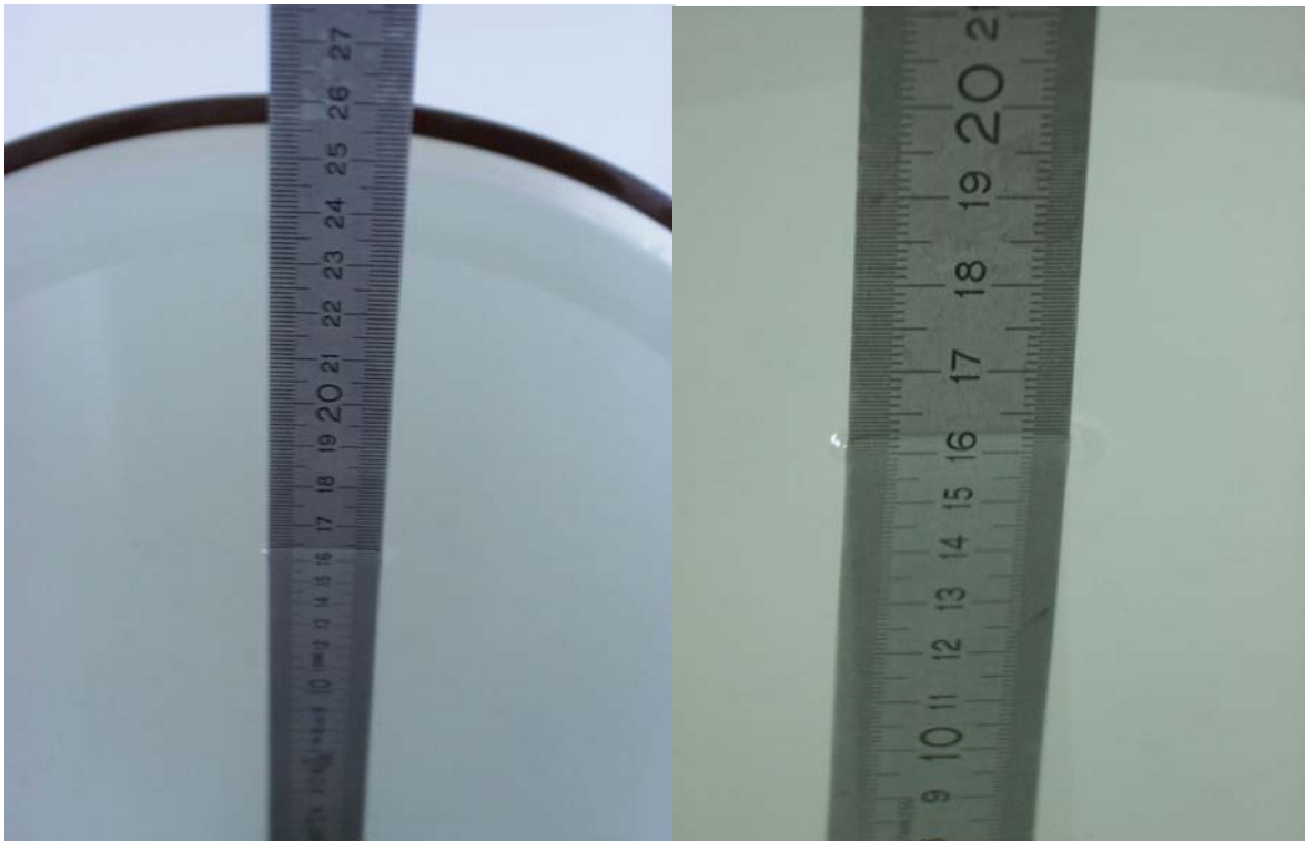
Fig. 41: Liquid depth for PCS 1900 head and body measurements.
