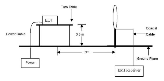
The diagram below shows the test setup that is utilized to make the measurements for emission from 30 Mz to 1 Gz emissions.
