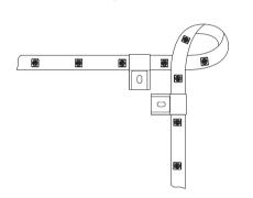
**Trimming the Strip:** The strip can be cut to a desired length at the designated marks. **Make sure the power adapter is unplugged before cutting.**
