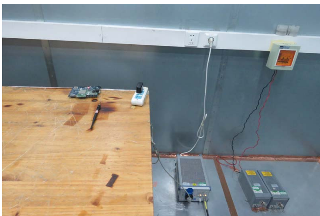
Picture 2 Conducted Emission Test Setup
