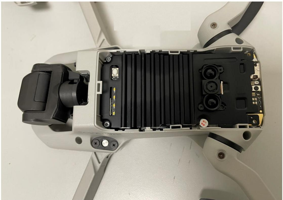
Figure 2: Internal view - 2 (with bottom cover removed)
