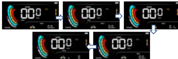
(4) 5-grid display of battery level: when the battery is full, the 5-grid lights are all on, and the battery flashes when the battery is under-voltage, indicating that it needs to be charged immediately. As shown below:
