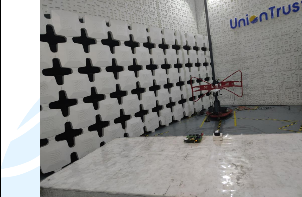
Radiated emission Test Setup-1 (30 MHz~1 GHz)
