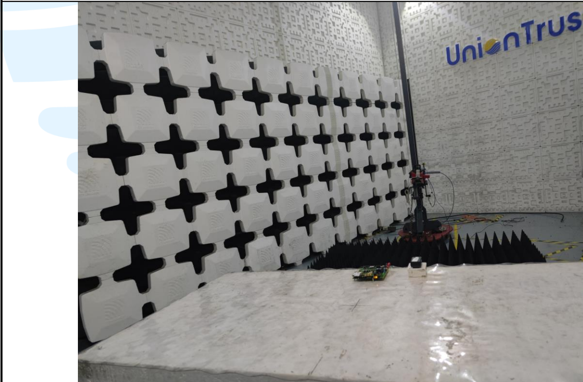
Radiated emission Test Setup-2 (Above 1 GHz)
