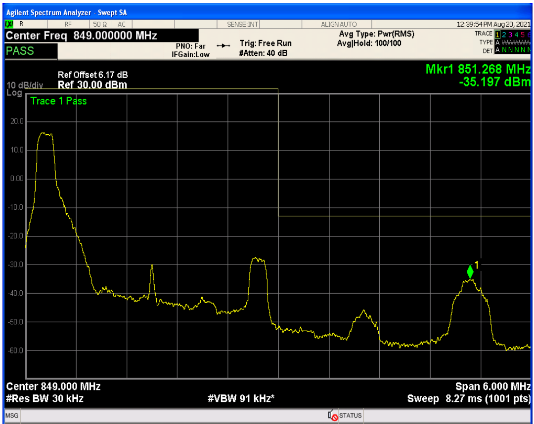
Band5 QAM16 BW=3MHz Channel=20415 RB Size=15 Position=#0
