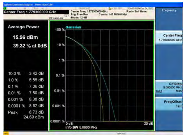
Band66 / 3MHz / Low CH / QPSK
