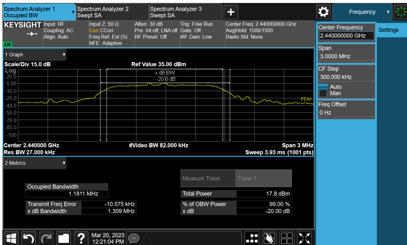
Figure TR42.1: Spectral data for Bluetooth EDR3 modulation at 2440 MHz
