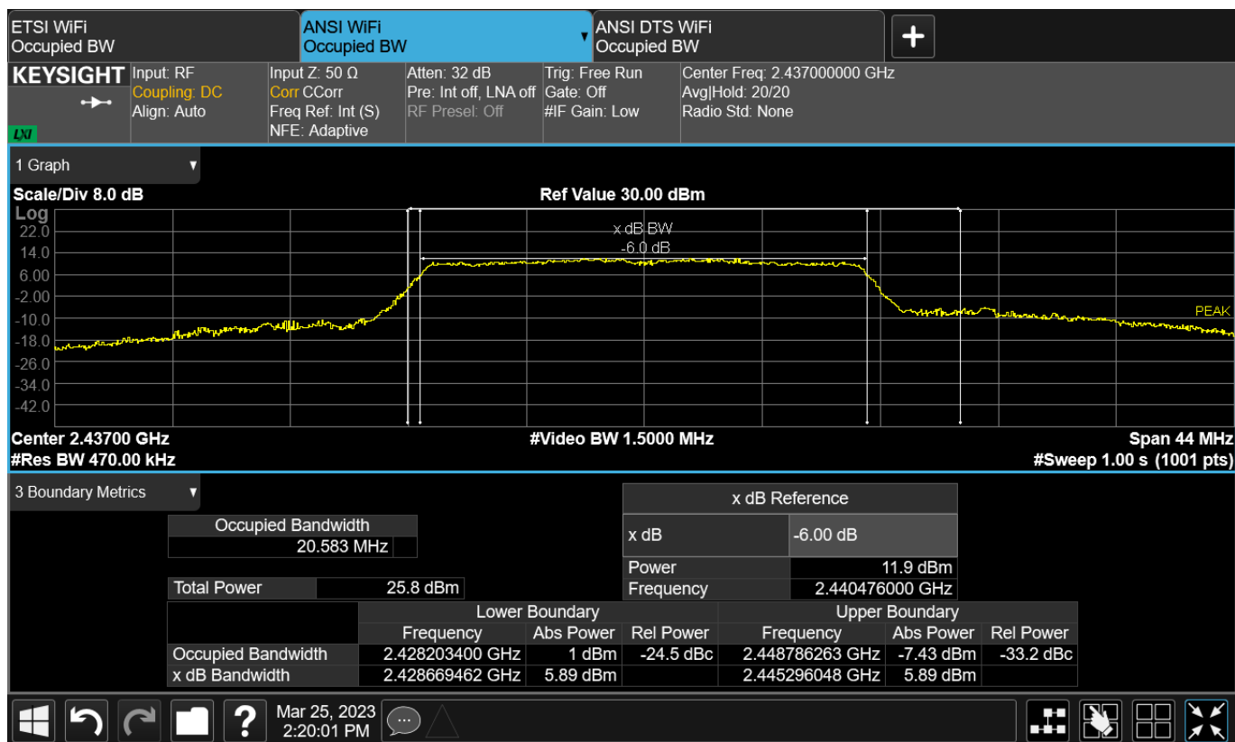
Figure TR15.5: Occupied bandwidth data for 802.11g 6 Mbps at channel 6
