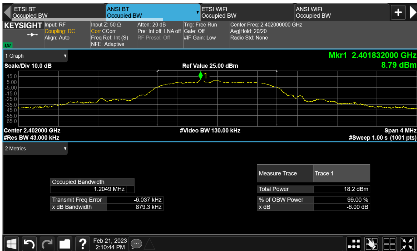
Figure TR15.1: Occupied bandwidth data for Bluetooth Classic EDR2 at low channel (2402 MHz)
