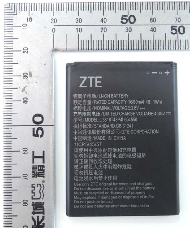
The battery view(Jiada Energy Technolog Co.,Ltd)
