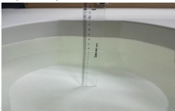
The Body Liquid of 2450MHz (15.3cm)
