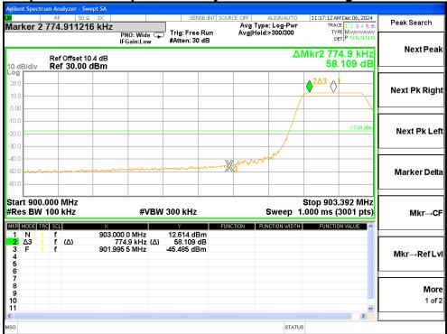
Screen Capture from the spectrum analyzer: Upper Band Edge
