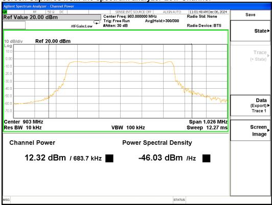
Screen Captures from the spectrum analyzer: MID Channel
