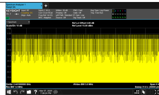
Number of Pulses in 31.6 seconds GFSK DH1
