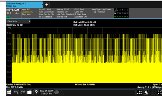
Number of Pulses in 31.6 seconds GFSK DH3
