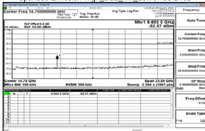
Spurious Emission High_BLE_1M_MidCH20-2442
