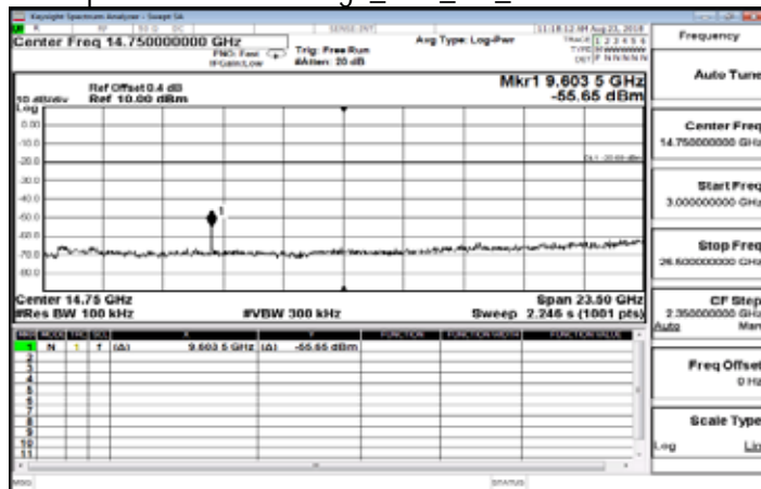
Spurious Emission High_BLE_2M_MidCH20-2442
