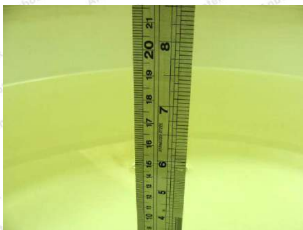
Photo of Liquid Height for Body SAR
