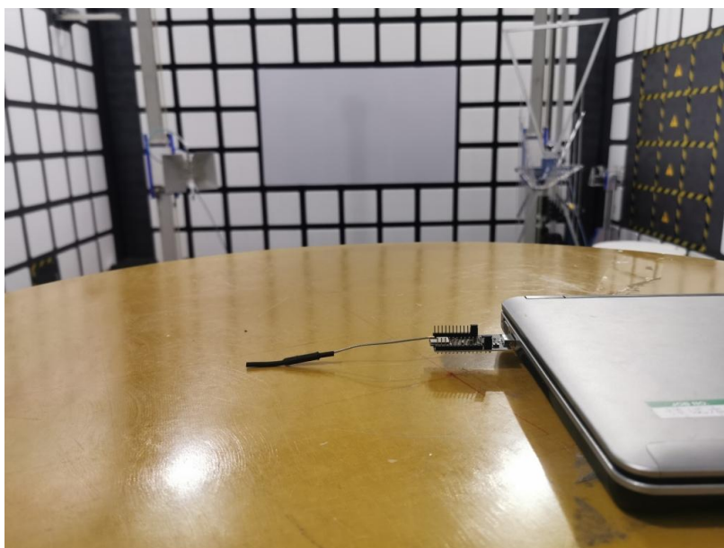
Spurious Radiated Emissions Test setup
