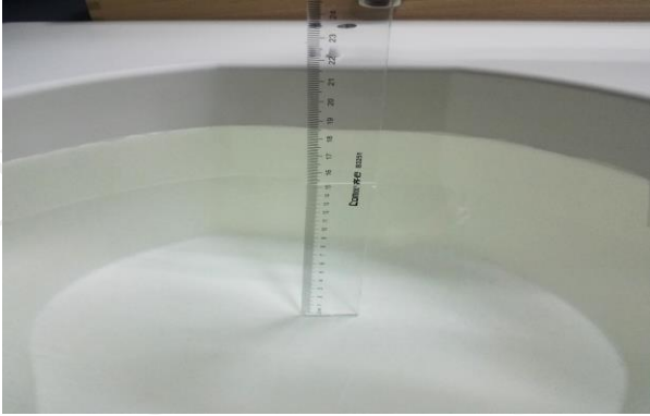
The Body Liquid of 2450MHz (15.3cm)
