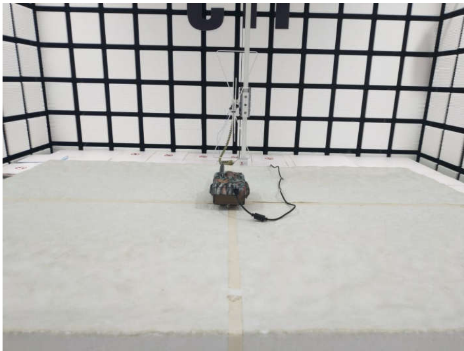
Radiated spurious emission Test Setup-1(Below 1GHz)
