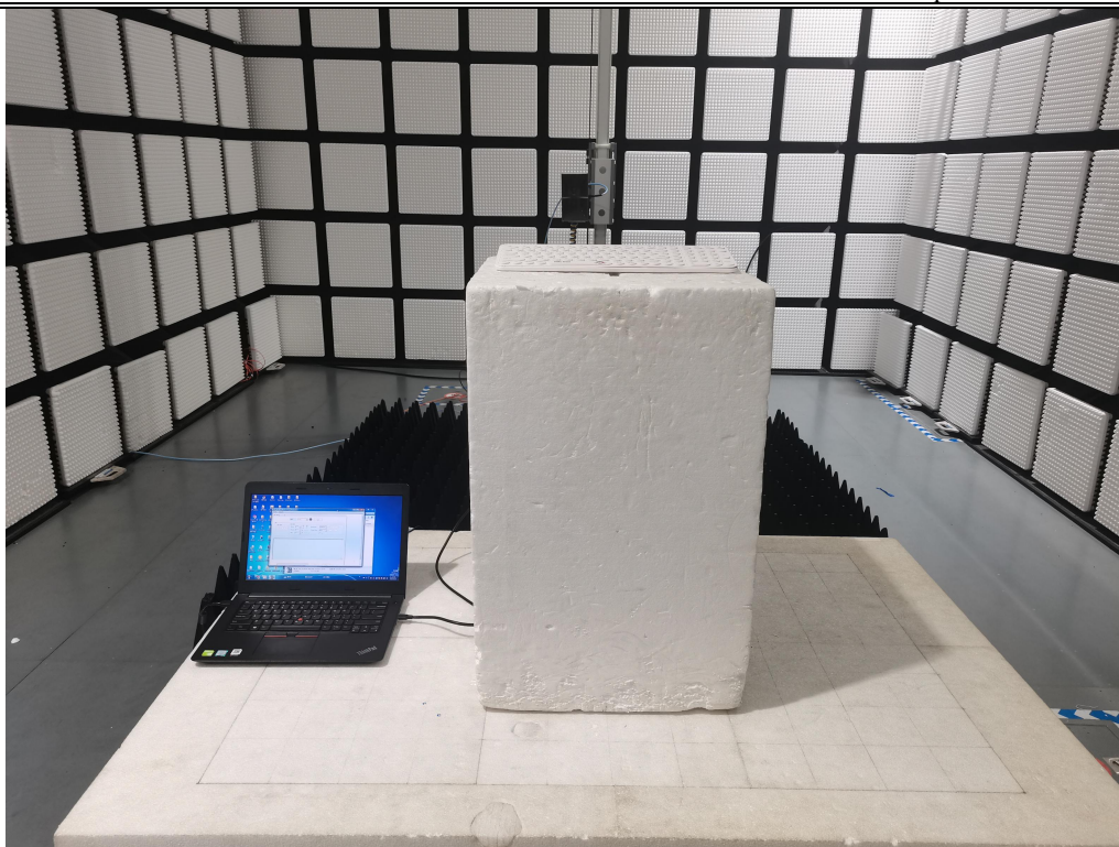
Fig. 3 Radiated emission setup photo(Above 1GHz)
