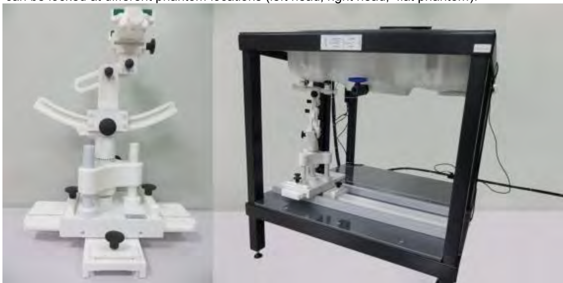
Device holder supplied by SATIMO
