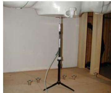
Figure 12.1 Dipole Validation Test Setup
