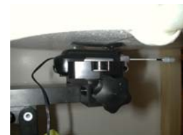
Figure 14.15 Body SAR Test Setup -- w/ Holster --
