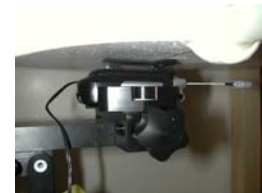
Figure 14.14 Body SAR Test Setup -- w/ Holster --
