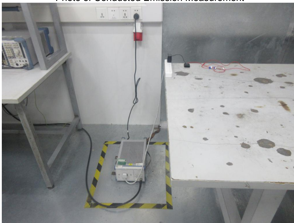
FCC ID: WSG-KH26 Photo of Conducted Emission Measurement
