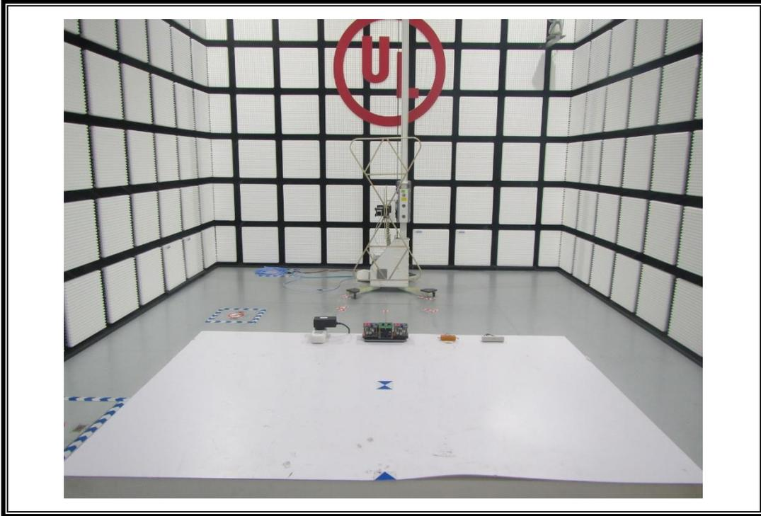
RADIATED EMISSIONS MEASUREMENT SETUP (30MHz ~ 1 GHz)
