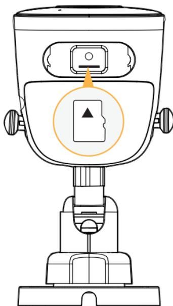
1. Remove the lower cover by unscrewing the Philips screws to access the SD card.
