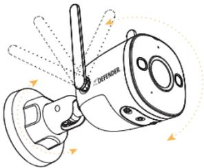
Loosen the adjustable joints and position the camera to ensure the best possible camera angle. Tighten the adjustable joints when finished.
