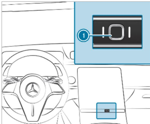
Fingerprint sensor ① allows you to conveniently access protected MBUX multimedia system functions and services. Compared to protection provided by the Mercedes me PIN, the entry of a four-digit number is not required to activate services and functions with personal content.
