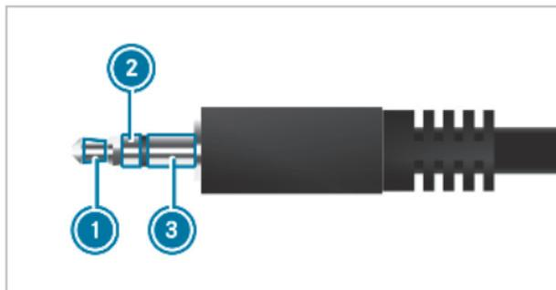
Example: connection of corded headphones with a 3-pin stereo jack, 3.5 mm
