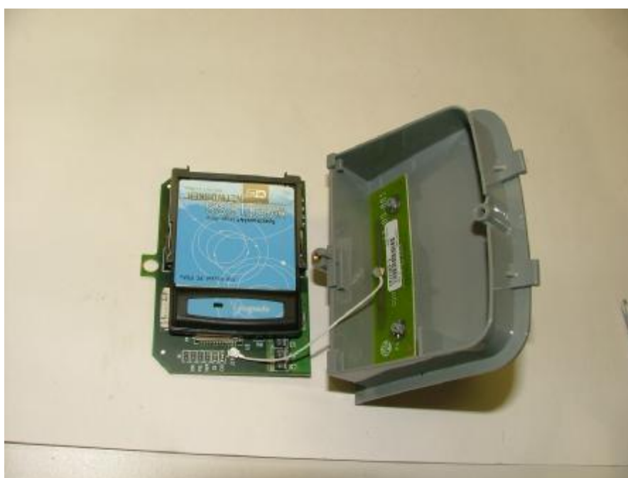
RF Carrier Board with H9PLA4137 and I28MD-BTC2TY4 Installed
