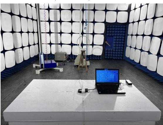
3. Radiated emission (9KHz-30MHz)
