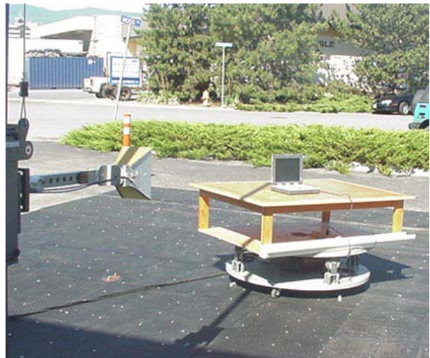
Photograph B.7-4 - Horn Substitution Setup
