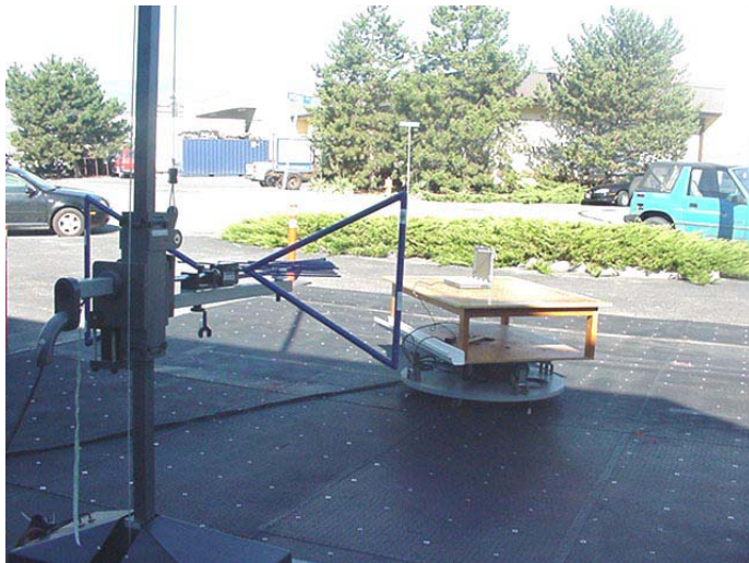
Photograph B.7-3 - Dipole Substitution Setup
