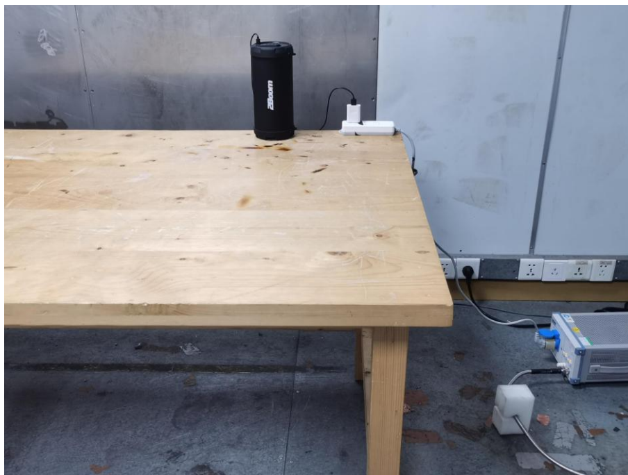
Photo of Power Line Conducted Emission Measurement
