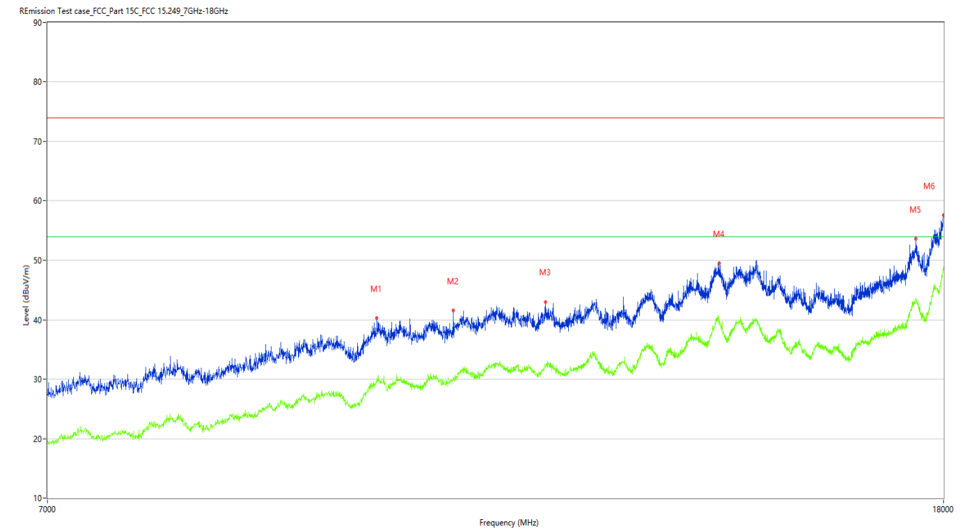
Figure 11: Test plots of Field strength of harmonics, 2403MHz, 7GHz-18GHz, Horizontal polarization
