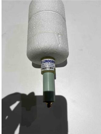
Fig 3 model 3126-5500 frequency 5500 MHz
