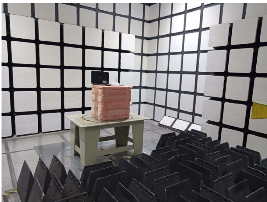
Radiated Emissions View (Above 1 GHz)
