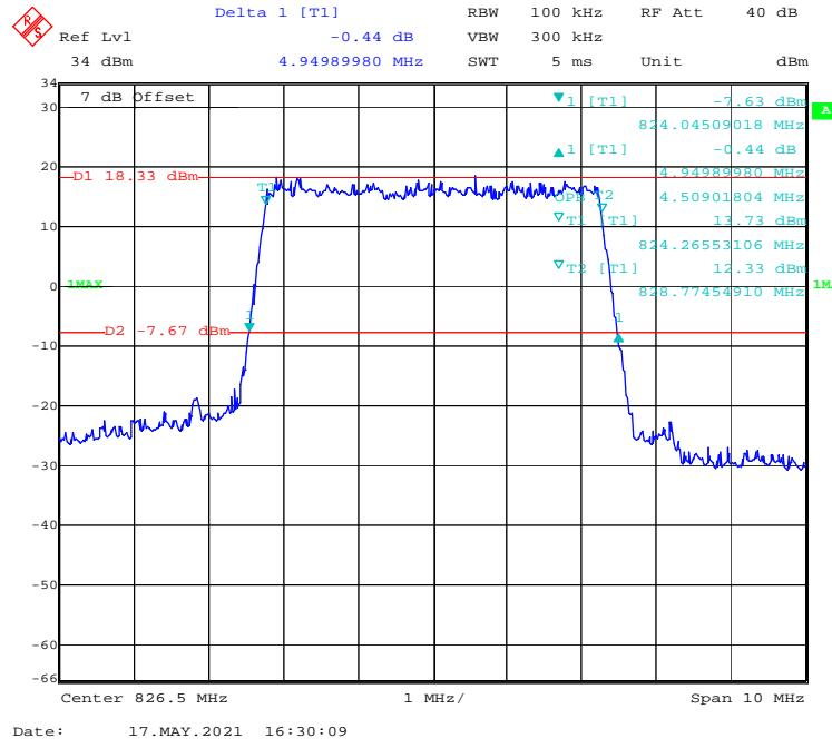
**QPSK (10.0 MHz) - 99% Occupied & 26 dB Emissions Bandwidth, Low channel**
