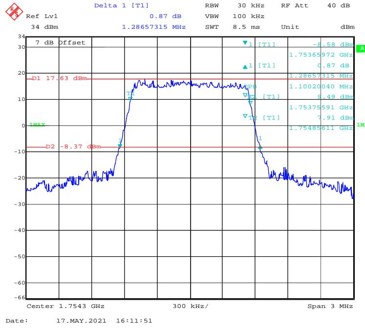
**16-QAM (3 MHz) - 99% Occupied & 26 dB Emissions Bandwidth, High channel**
