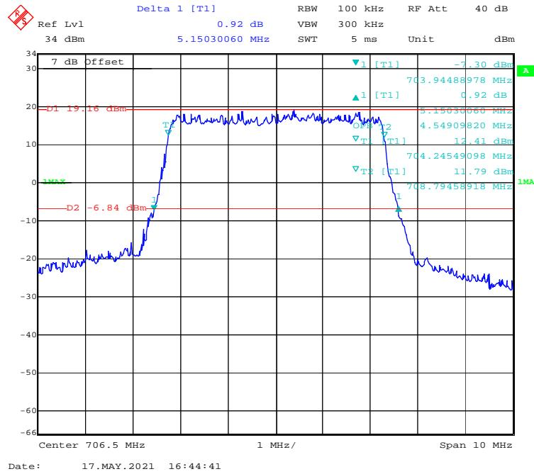
**16-QAM (10 MHz) - 99% Occupied & 26 dB Emissions Bandwidth, Low channel**
