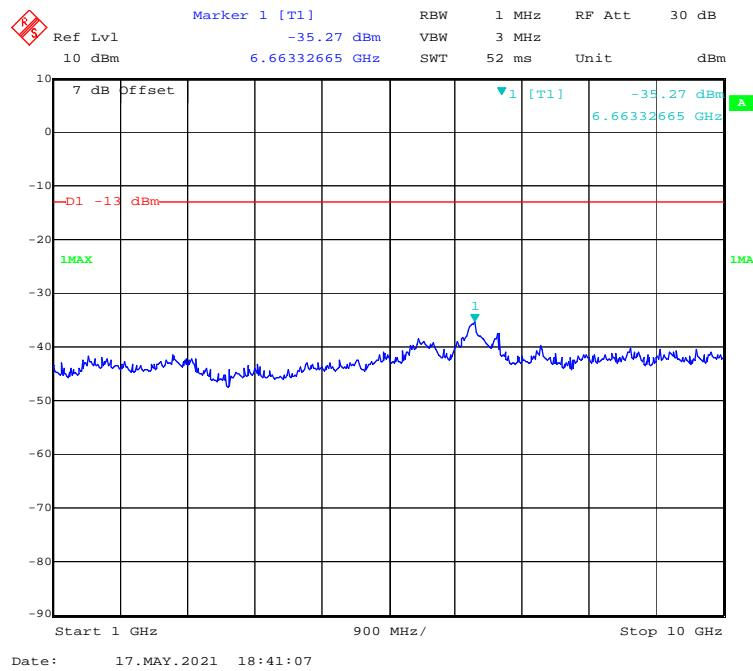
**30 MHz - 1 GHz (QPSK, 10.0 MHz, Middle Channel)**
