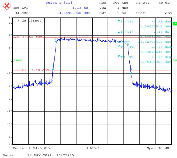
**16-QAM (20 MHz) - 99% Occupied & 26 dB Emissions Bandwidth, High channel**
