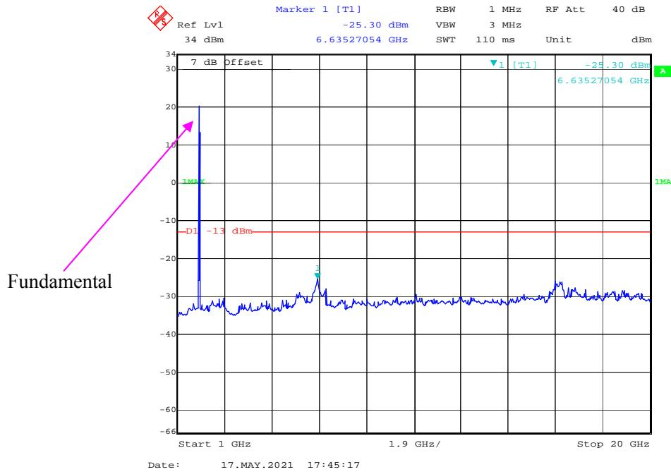
**30 MHz - 1 GHz (20 MHz, QPSK, High Channel)**
