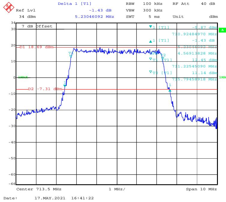
**16-QAM (10 MHz) - 99% Occupied & 26 dB Emissions Bandwidth, High channel**
