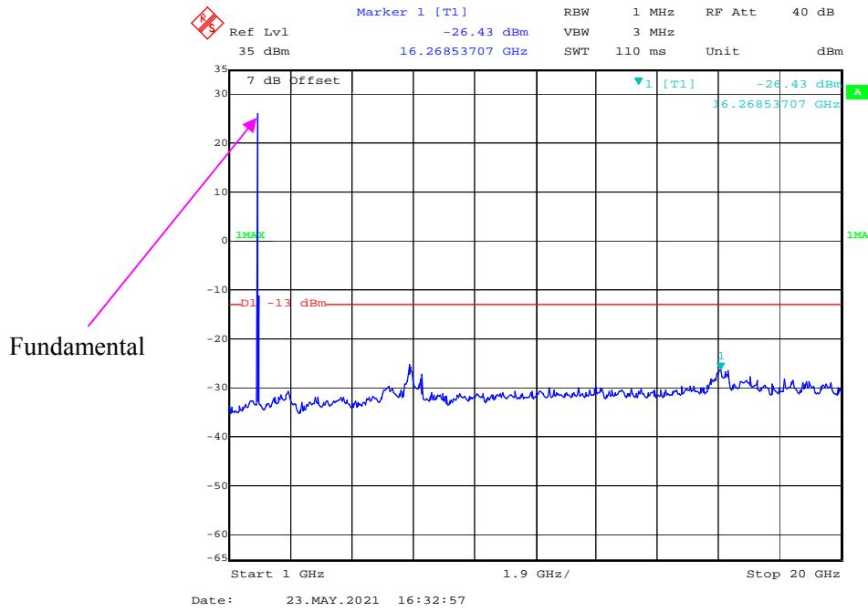
**30 MHz – 1GHz WCDMA (HSPA+) Mode , High channel**
