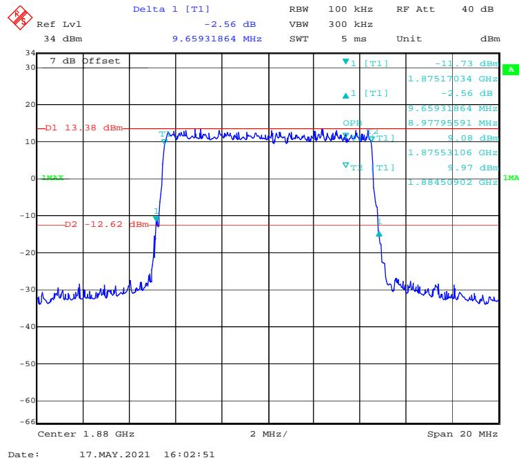
**16-QAM (15 MHz) - 99% Occupied & 26 dB Emissions Bandwidth, Middle channel**
