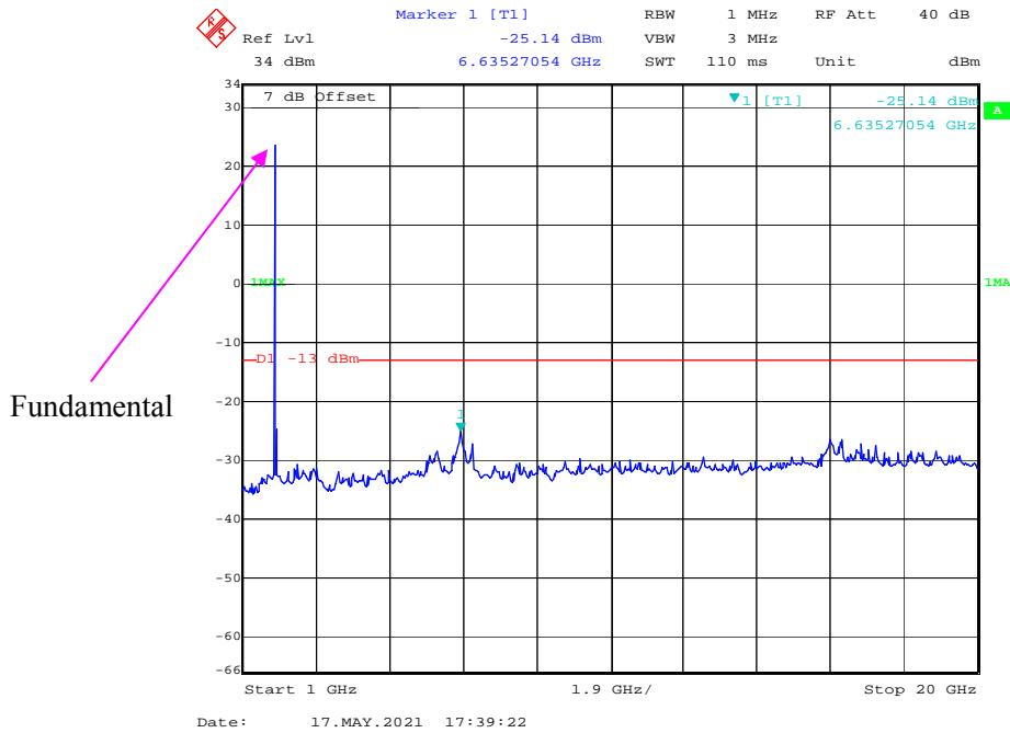
**30 MHz - 1 GHz (5 MHz, QPSK, Low Channel)**
