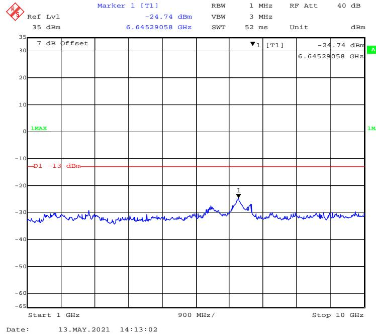
**30 MHz – 1GHz WCDMA (HSUPA) Mode, High channel**
