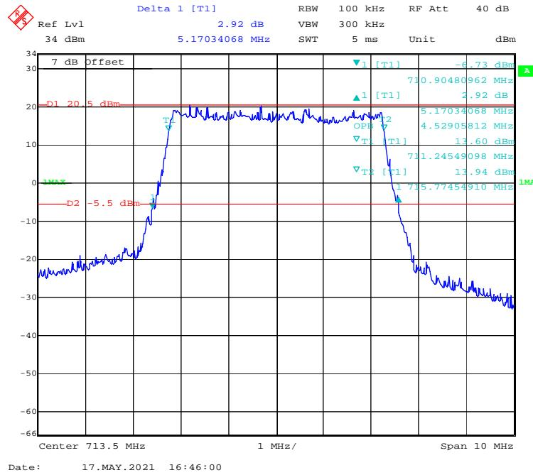
**QPSK (10MHz) - 99% Occupied & 26 dB Emissions Bandwidth, High channel**
