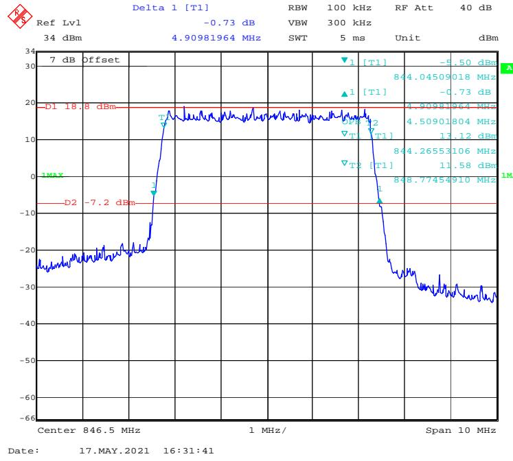
**QPSK (10.0 MHz) - 99% Occupied & 26 dB Emissions Bandwidth, High channel**
