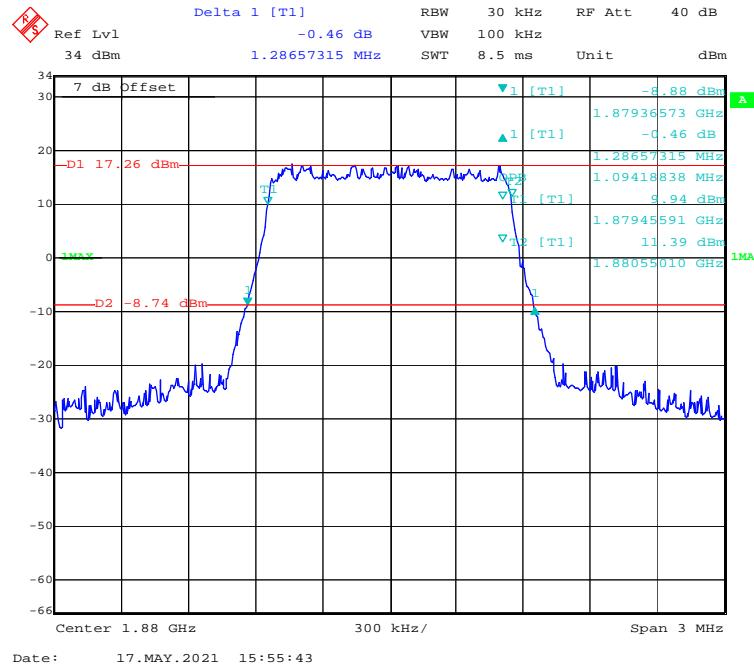
**16-QAM (3 MHz) - 99% Occupied & 26 dB Emissions Bandwidth, Middle channel**
