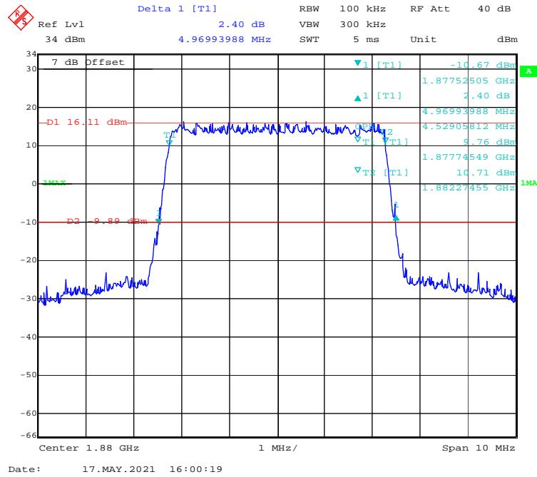
**16-QAM (10 MHz) - 99% Occupied & 26 dB Emissions Bandwidth, Middle channel**
