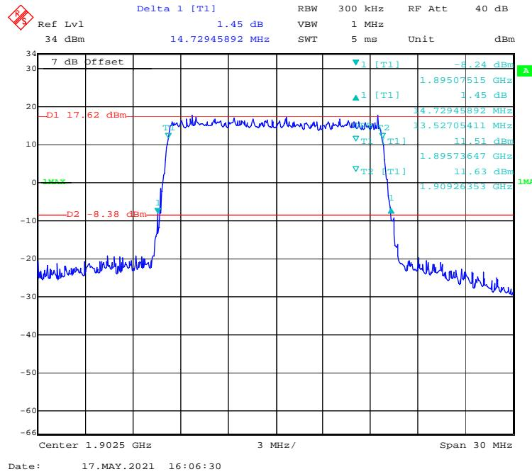
**16-QAM (20 MHz) - 99% Occupied & 26 dB Emissions Bandwidth, High channel**
