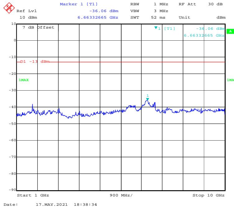
**30 MHz - 1 GHz (QPSK, 3.0 MHz, High Channel)**
