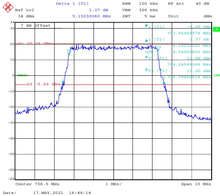
**QPSK (10MHz) - 99% Occupied & 26 dB Emissions Bandwidth, Low channel**
