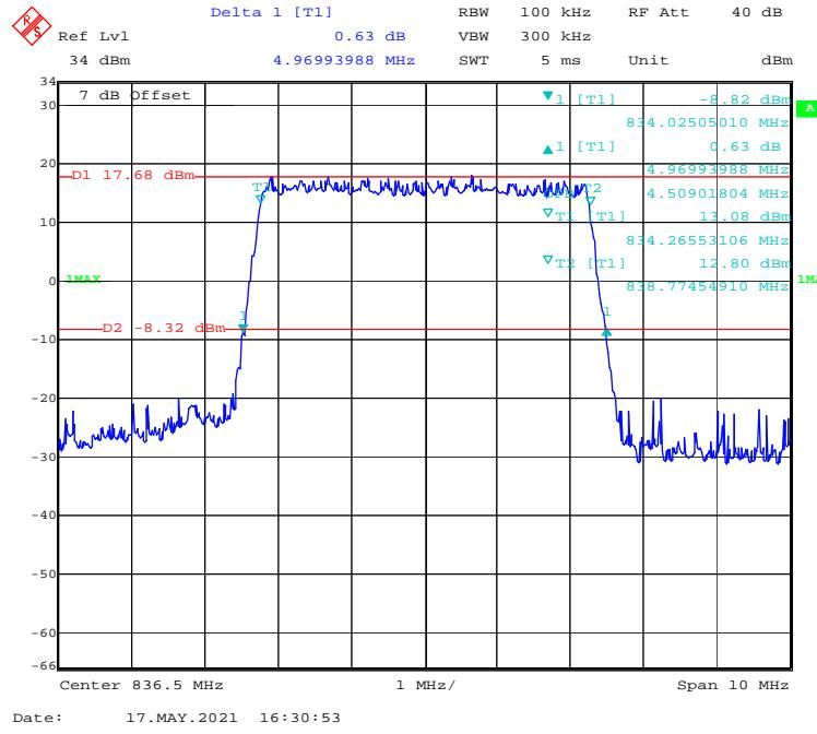
**QPSK (10.0 MHz) - 99% Occupied & 26 dB Emissions Bandwidth, Middle channel**
