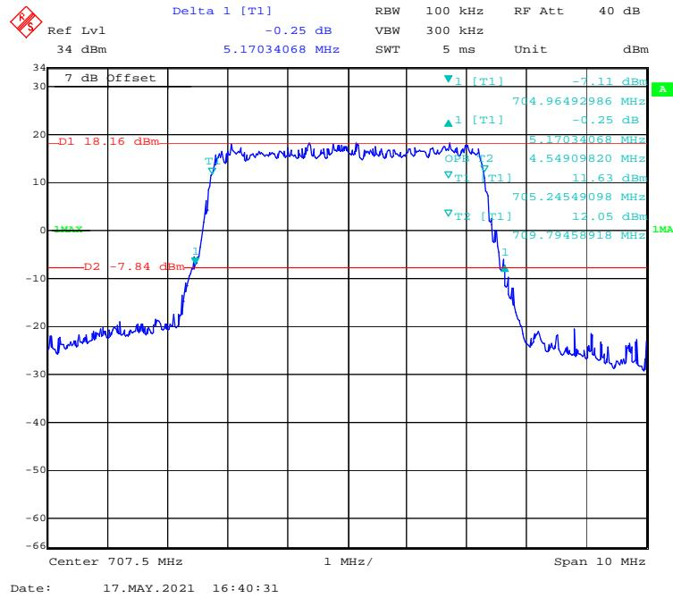
**16-QAM (10 MHz) - 99% Occupied & 26 dB Emissions Bandwidth, Middle channel**
