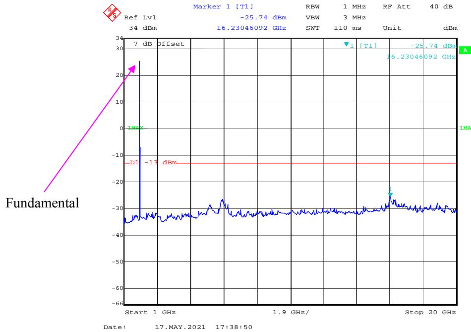
**30 MHz - 1 GHz (3 MHz, QPSK, High Channel)**
