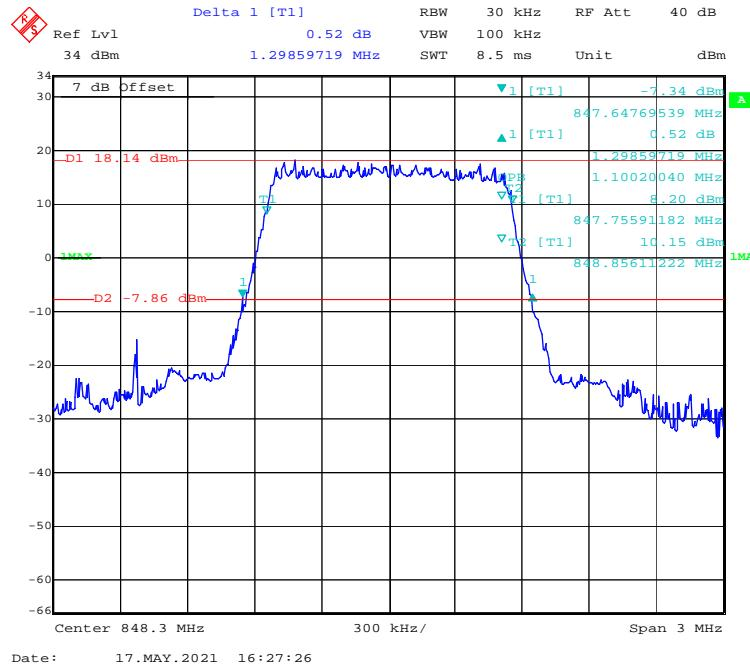
**16-QAM (3.0 MHz) - 99% Occupied & 26 dB Emissions Bandwidth, High channel**
