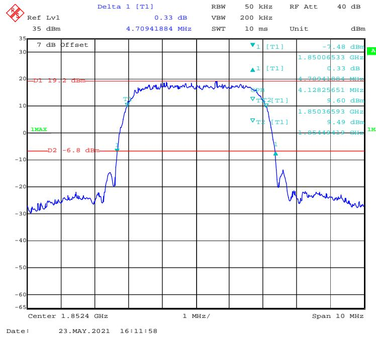
**99% Occupied & 26 dB Emissions Bandwidth for WCDMA (HSPA+) Middle channel**
