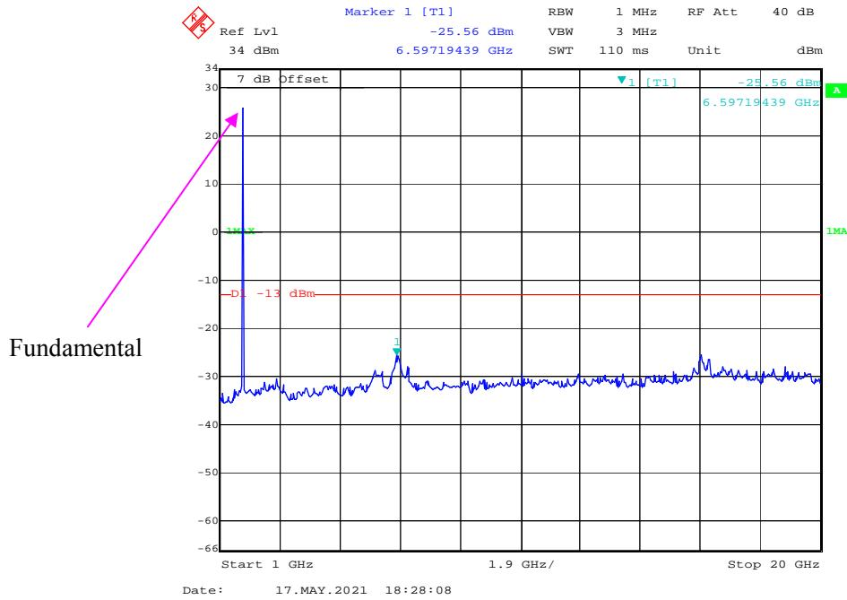
**30 MHz - 1 GHz (1.4 MHz, 16-QAM, Middle Channel)**
