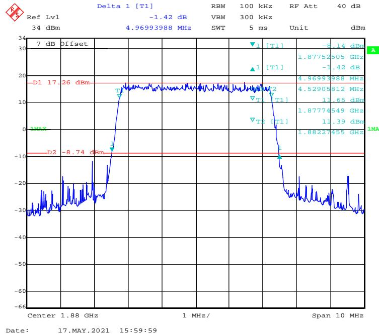
**QPSK (10MHz) - 99% Occupied & 26 dB Emissions Bandwidth, Middle channel**
