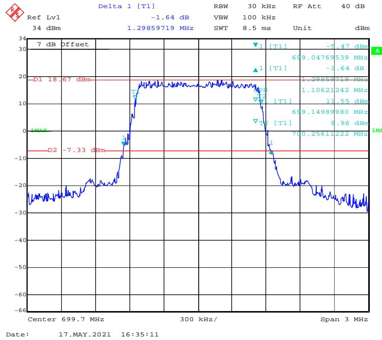
**16-QAM (3 MHz) - 99% Occupied & 26 dB Emissions Bandwidth, Low channel**
