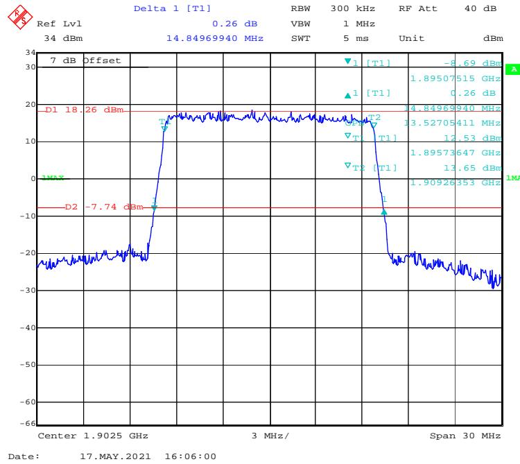
**QPSK (20 MHz) - 99% Occupied & 26 dB Emissions Bandwidth, High channel**
