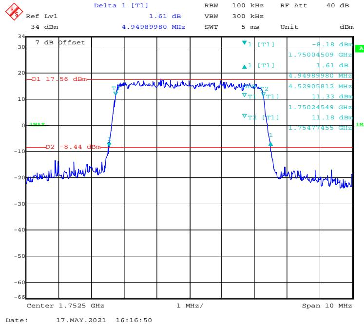
**16-QAM (10 MHz) - 99% Occupied & 26 dB Emissions Bandwidth, High channel**
