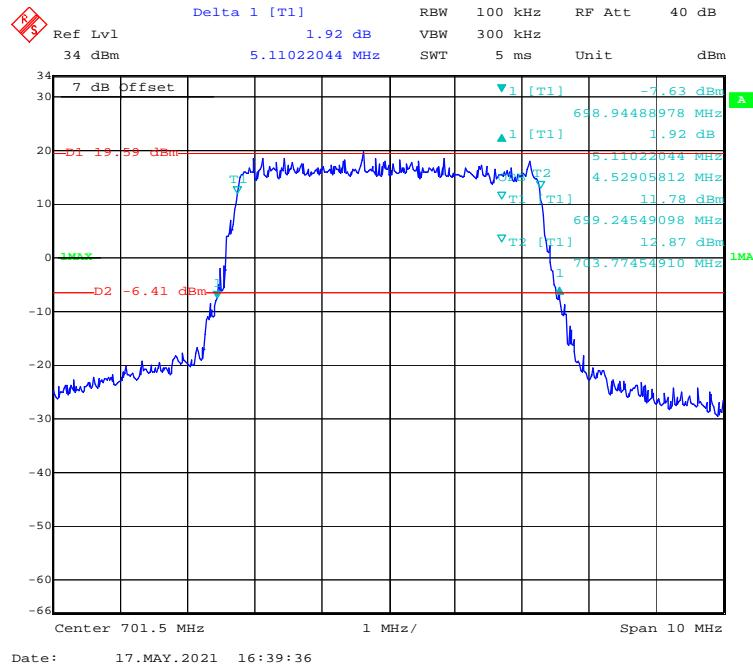
**16-QAM (10 MHz) - 99% Occupied & 26 dB Emissions Bandwidth, Low channel**
