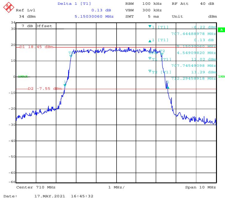
**16-QAM (10 MHz) - 99% Occupied & 26 dB Emissions Bandwidth, Middle channel**
