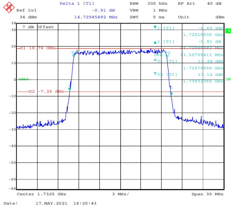
**QPSK (20 MHz) - 99% Occupied & 26 dB Emissions Bandwidth, Middle channel**
