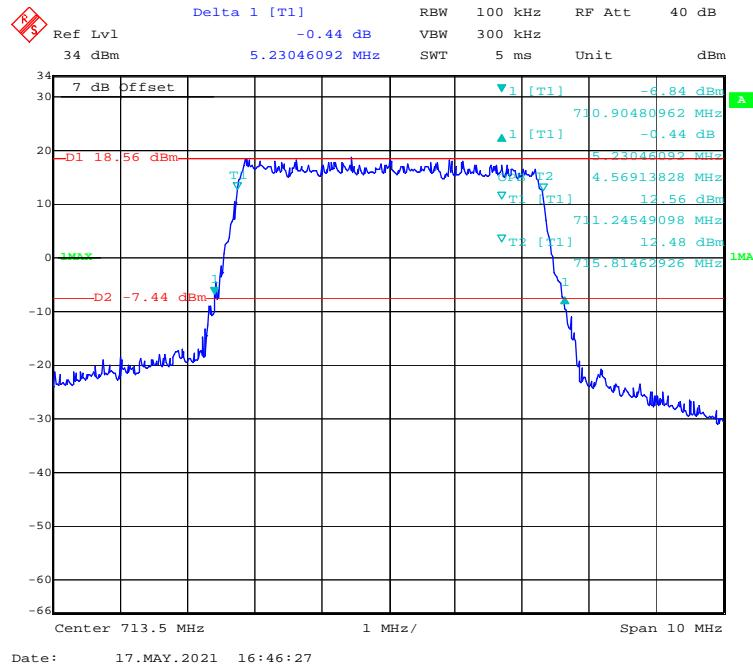
**16-QAM (10 MHz) - 99% Occupied & 26 dB Emissions Bandwidth, High channel**
