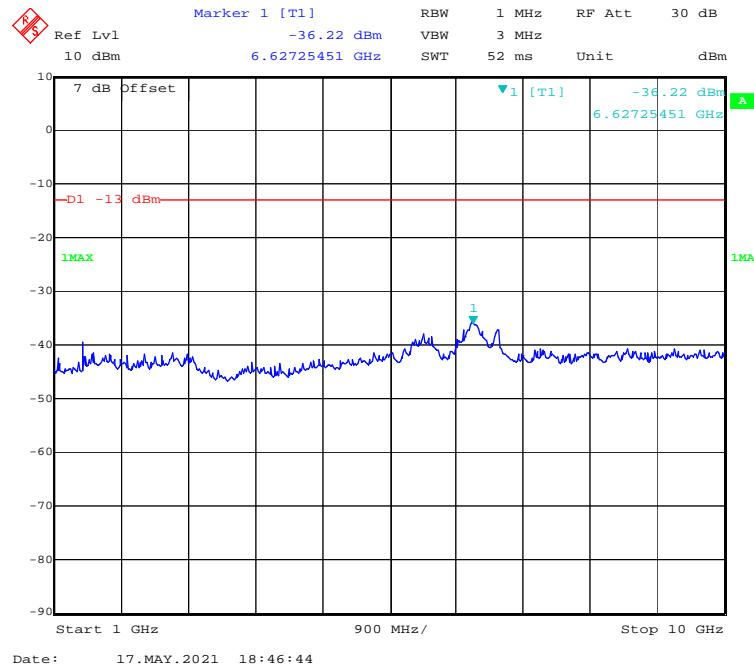
**30 MHz - 1 GHz (5 MHz, 16-QAM, Low Channel)**
