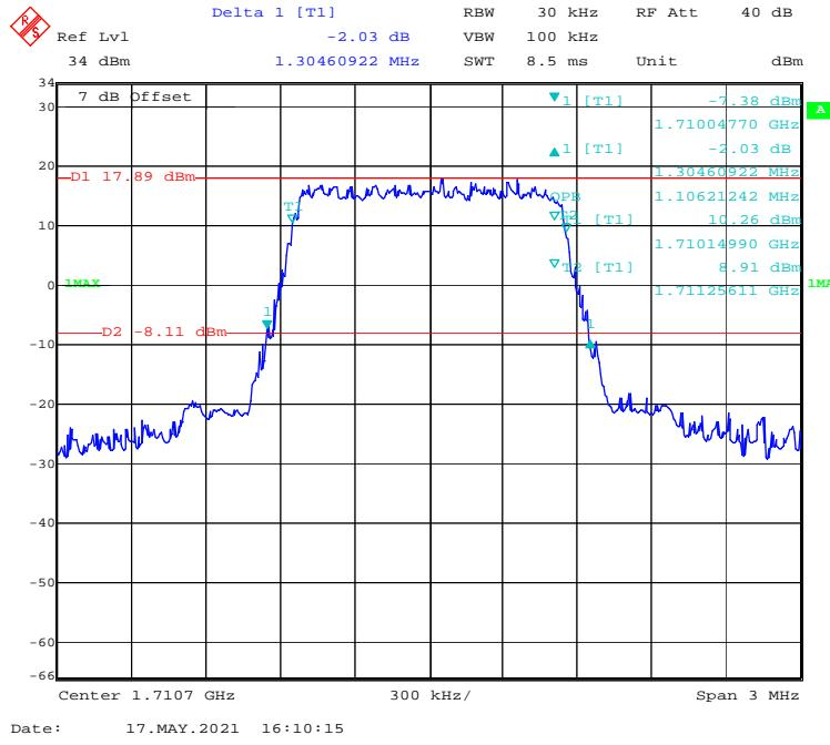
**16-QAM (3 MHz) - 99% Occupied & 26 dB Emissions Bandwidth, Low channel**
