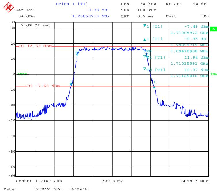
**QPSK (3 MHz) - 99% Occupied & 26 dB Emissions Bandwidth, Low channel**
