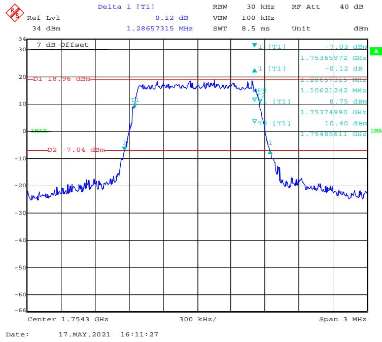
**QPSK (3 MHz) - 99% Occupied & 26 dB Emissions Bandwidth, High channel**
