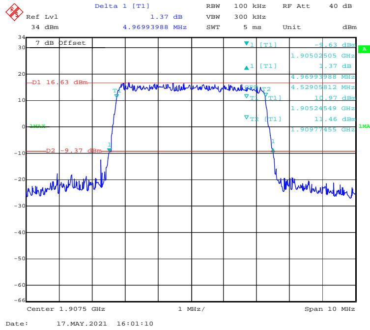
**16-QAM (10 MHz) - 99% Occupied & 26 dB Emissions Bandwidth, High channel**
