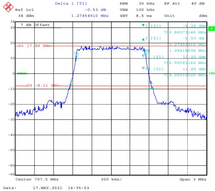
**16-QAM (3 MHz) - 99% Occupied & 26 dB Emissions Bandwidth, Middle channel**
