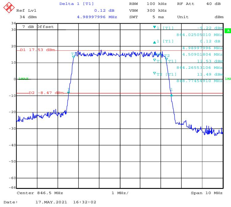
**16-QAM (10.0 MHz) - 99% Occupied & 26 dB Emissions Bandwidth, High channel**
