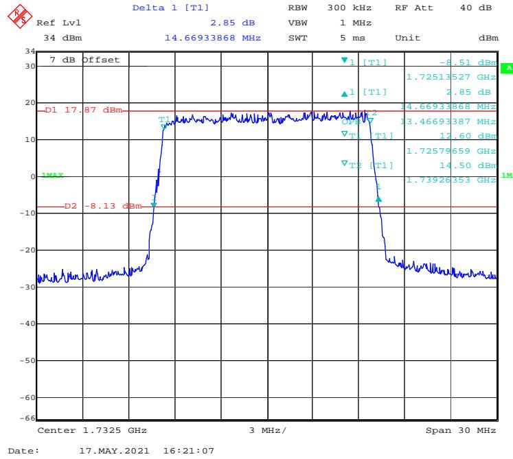
**16-QAM (20 MHz) - 99% Occupied & 26 dB Emissions Bandwidth, Middle channel**
