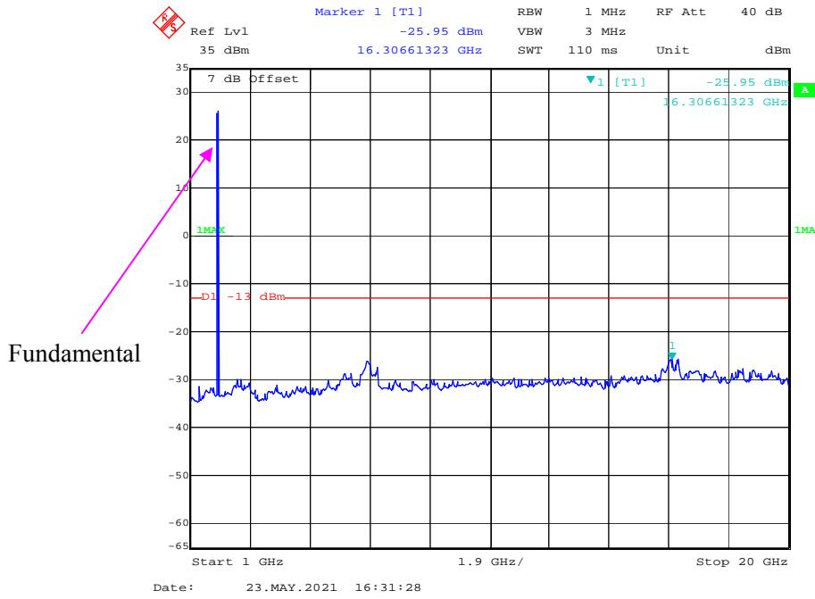
**30 MHz – 1GHz WCDMA (Rel 99) Mode , High channel**
