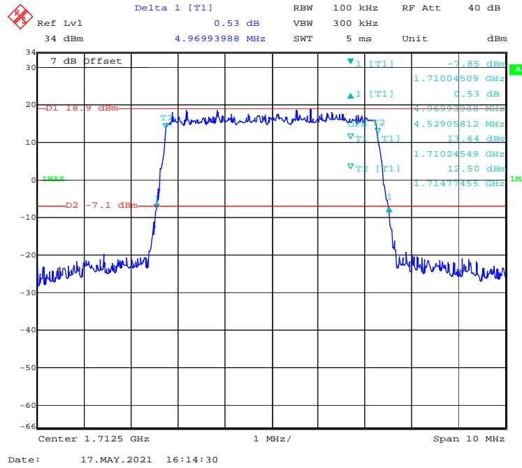
**QPSK (10 MHz) - 99% Occupied & 26 dB Emissions Bandwidth, Low channel**
