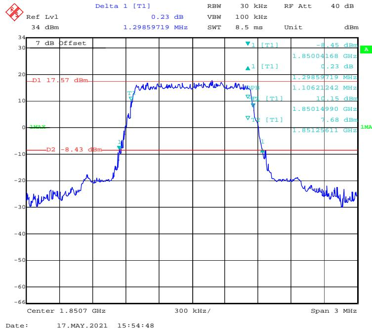
**16-QAM (3 MHz) - 99% Occupied & 26 dB Emissions Bandwidth, Low channel**
