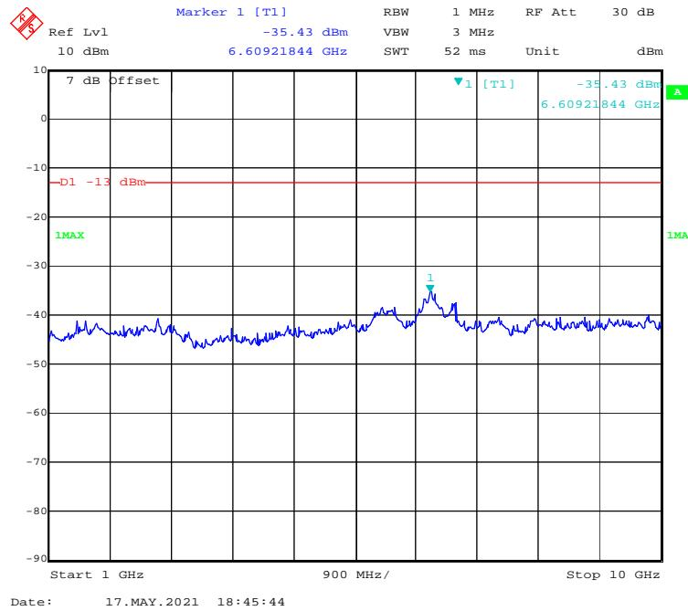
**30 MHz - 1 GHz (3 MHz, 16-QAM, Middle Channel)**
