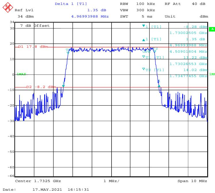
**QPSK (10 MHz) - 99% Occupied & 26 dB Emissions Bandwidth, Middle channel**
