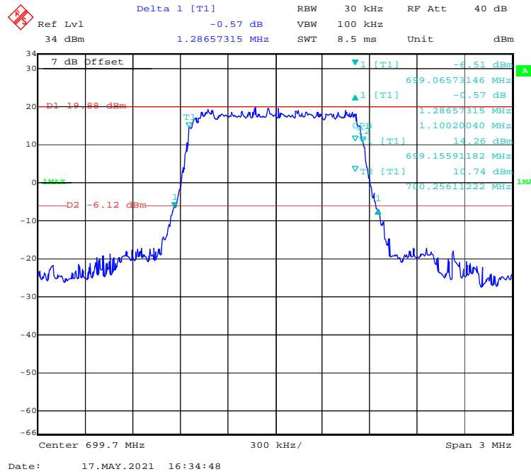
**QPSK (3 MHz) - 99% Occupied & 26 dB Emissions Bandwidth, Low channel**
