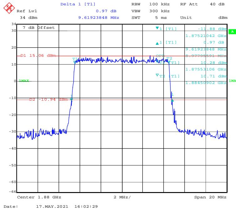
**QPSK (15 MHz) - 99% Occupied & 26 dB Emissions Bandwidth, Middle channel**
