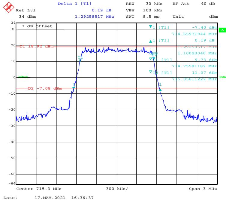
**16-QAM (3 MHz) - 99% Occupied & 26 dB Emissions Bandwidth, High channel**
