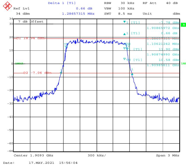
**QPSK (3 MHz) - 99% Occupied & 26 dB Emissions Bandwidth, High channel**
