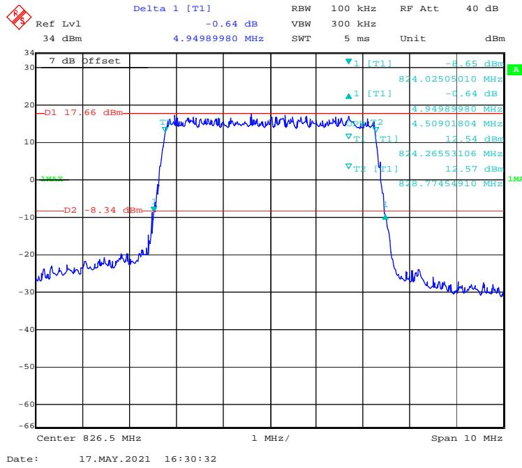
**16-QAM (10.0 MHz) - 99% Occupied & 26 dB Emissions Bandwidth, Low channel**
