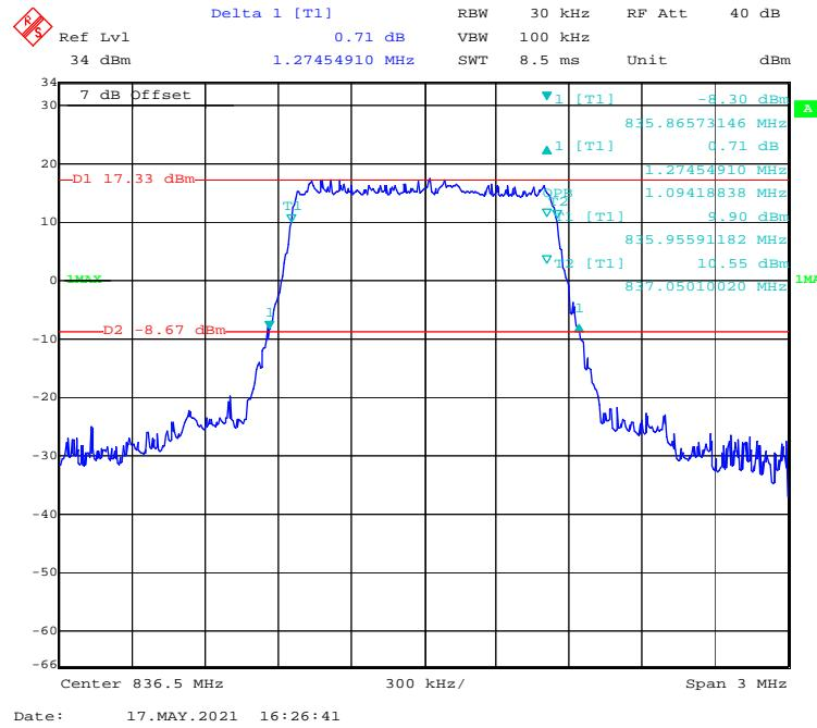
**16-QAM (3.0 MHz) - 99% Occupied & 26 dB Emissions Bandwidth, Middle channel**
