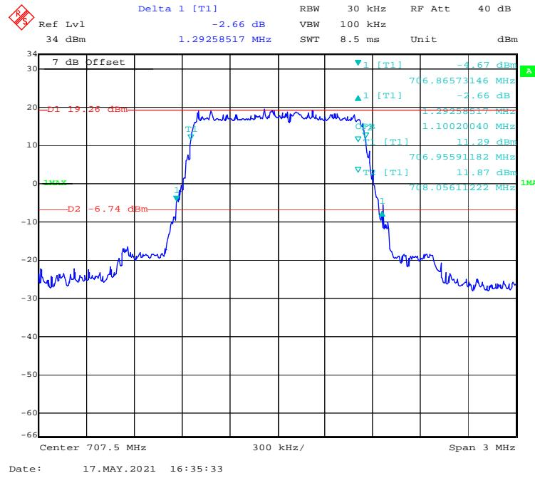
**QPSK (3 MHz) - 99% Occupied & 26 dB Emissions Bandwidth, Middle channel**
