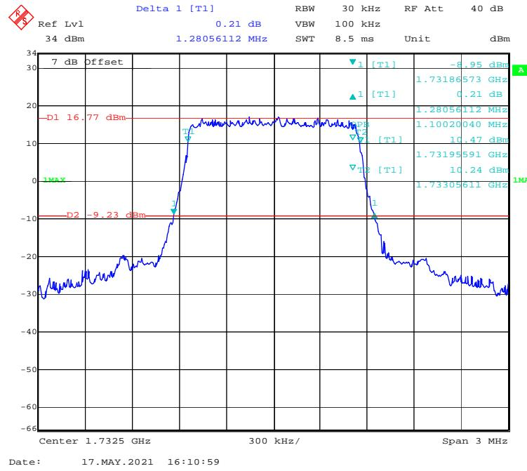
**16-QAM (3 MHz) - 99% Occupied & 26 dB Emissions Bandwidth, Middle channel**
