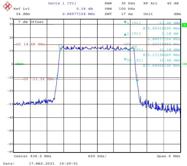
**16-QAM (5.0 MHz) - 99% Occupied & 26 dB Emissions Bandwidth, Middle channel**
