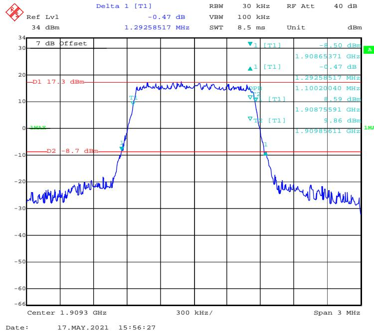
**16-QAM (3 MHz) - 99% Occupied & 26 dB Emissions Bandwidth, High channel**
