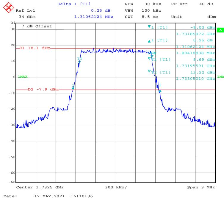
**QPSK (3 MHz) - 99% Occupied & 26 dB Emissions Bandwidth, Middle channel**
