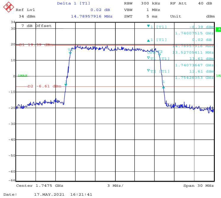
**QPSK (20 MHz) - 99% Occupied & 26 dB Emissions Bandwidth, High channel**
