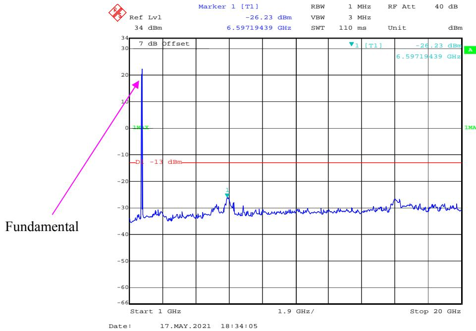
**30 MHz - 1 GHz (15 MHz, 16-QAM, Low Channel)**
