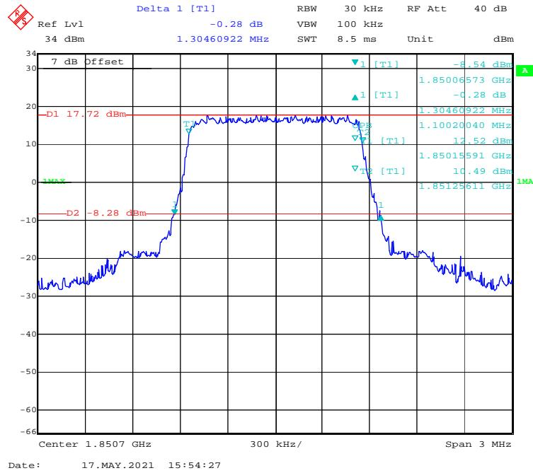
**QPSK (3 MHz) - 99% Occupied & 26 dB Emissions Bandwidth, Low channel**
