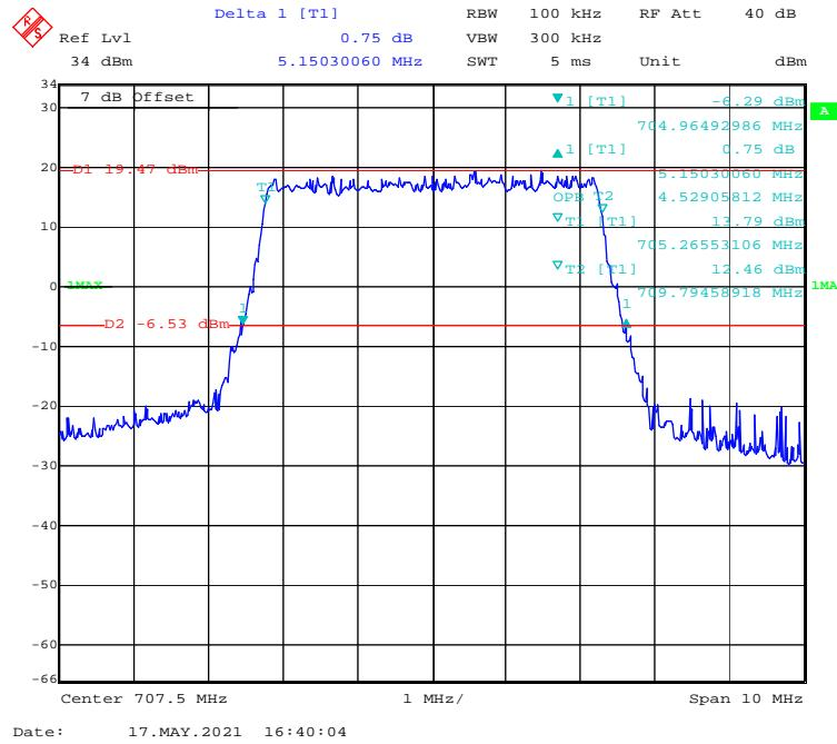
**QPSK (10MHz) - 99% Occupied & 26 dB Emissions Bandwidth, Middle channel**
