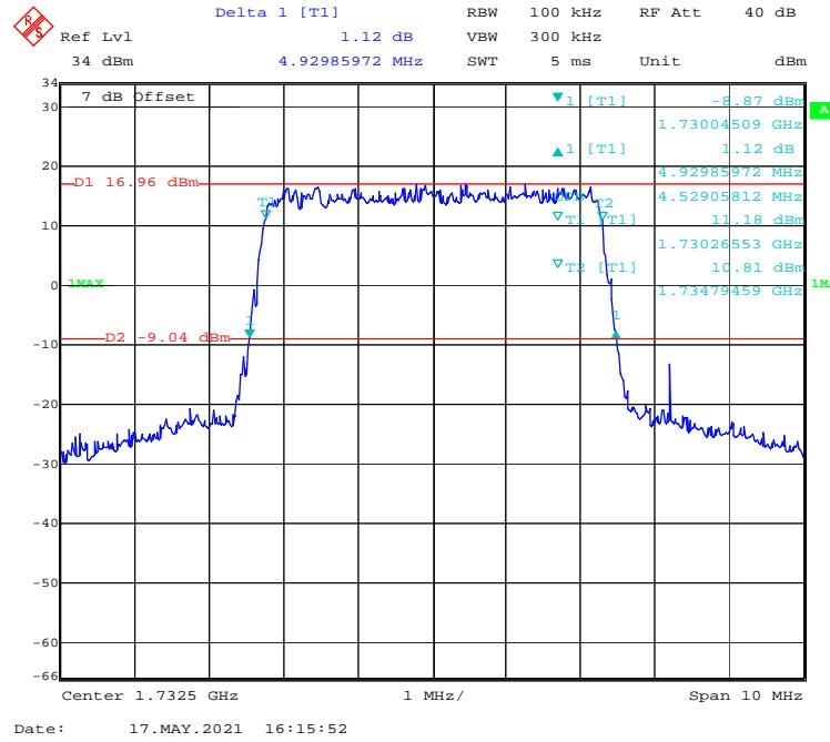
**16-QAM (10 MHz) - 99% Occupied & 26 dB Emissions Bandwidth, Middle channel**
