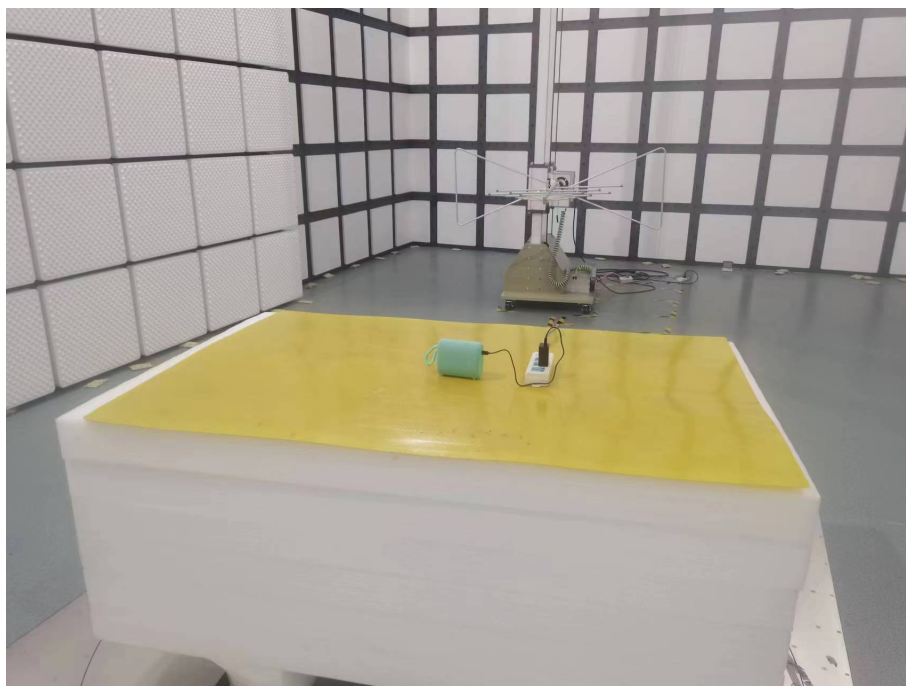
Photo of Radiated Emission Measurement (Above 1G)
